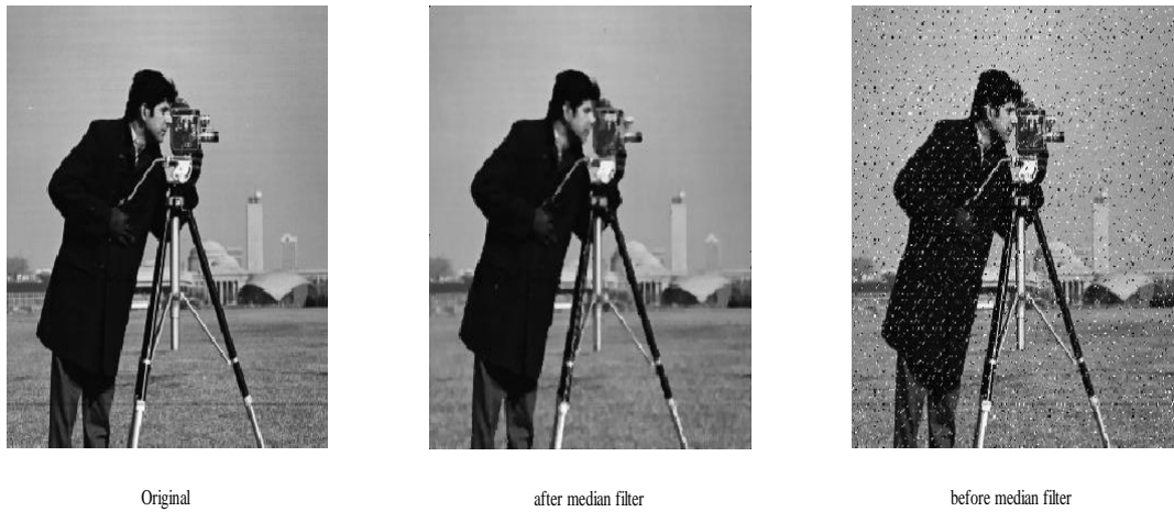
Figure 5.10: Image Transmission with 64-QAM through RA6 Channel at 24 dB
