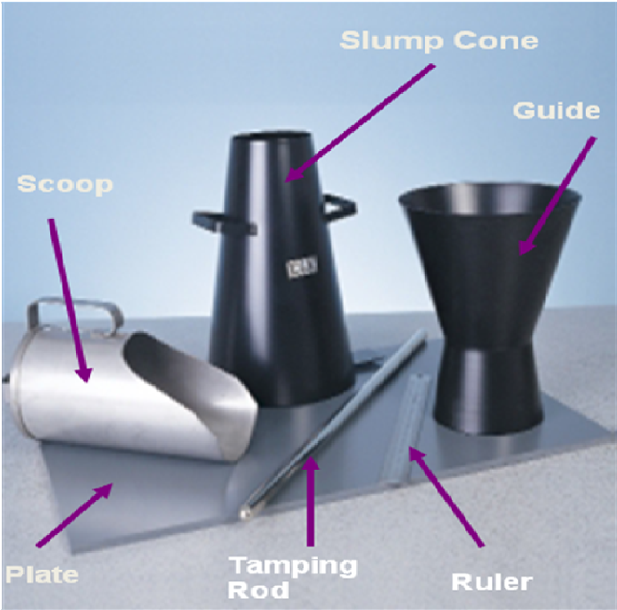
Figure 3. Slump cone test.
