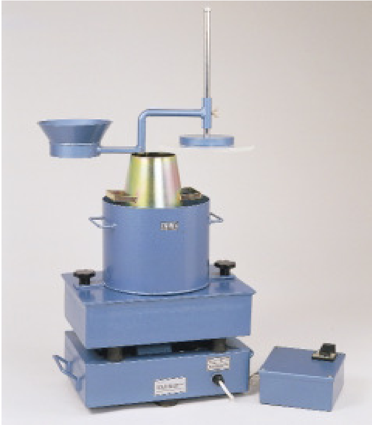
Figure 2. VeBe consistometer test.
