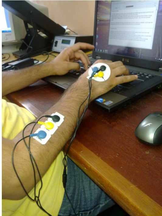
Figure 3.1: Placement of sEMG electrodes on hand (musculi lumbricales manus) and forearm (extensor carpi radialis)
