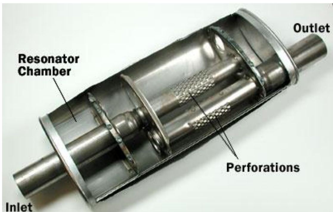
Figure 2. A typical reactive muffler for automotive application [1]
