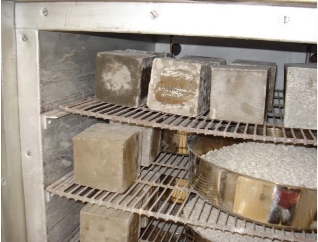
Photo 3.17: Samples were Placed in Oven to Obtain Oven-Dry Condition.
