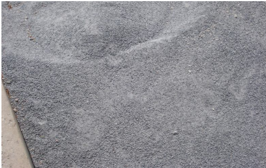
Photo 3.5: Limestone Aggregate (size \leq 2 mm)
