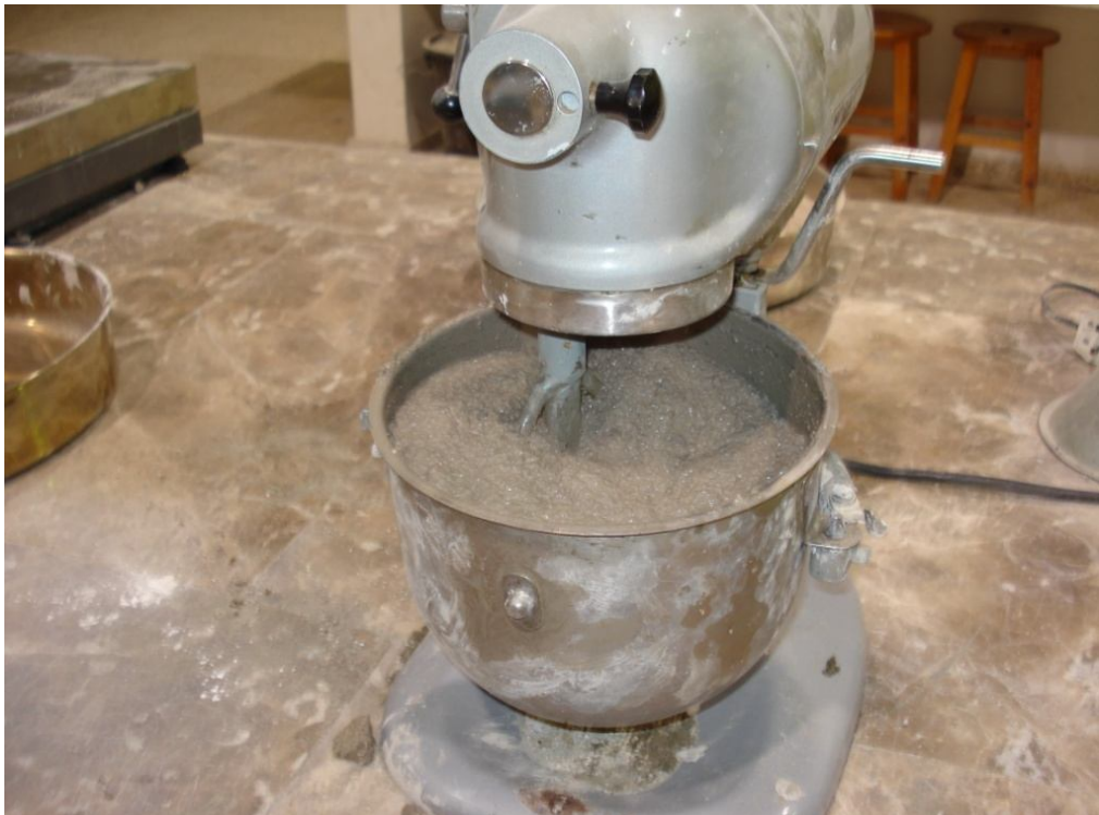
Photo 3.9: Mortar was Mixed by Mortar Mixer for Prepare Test Specimens.
