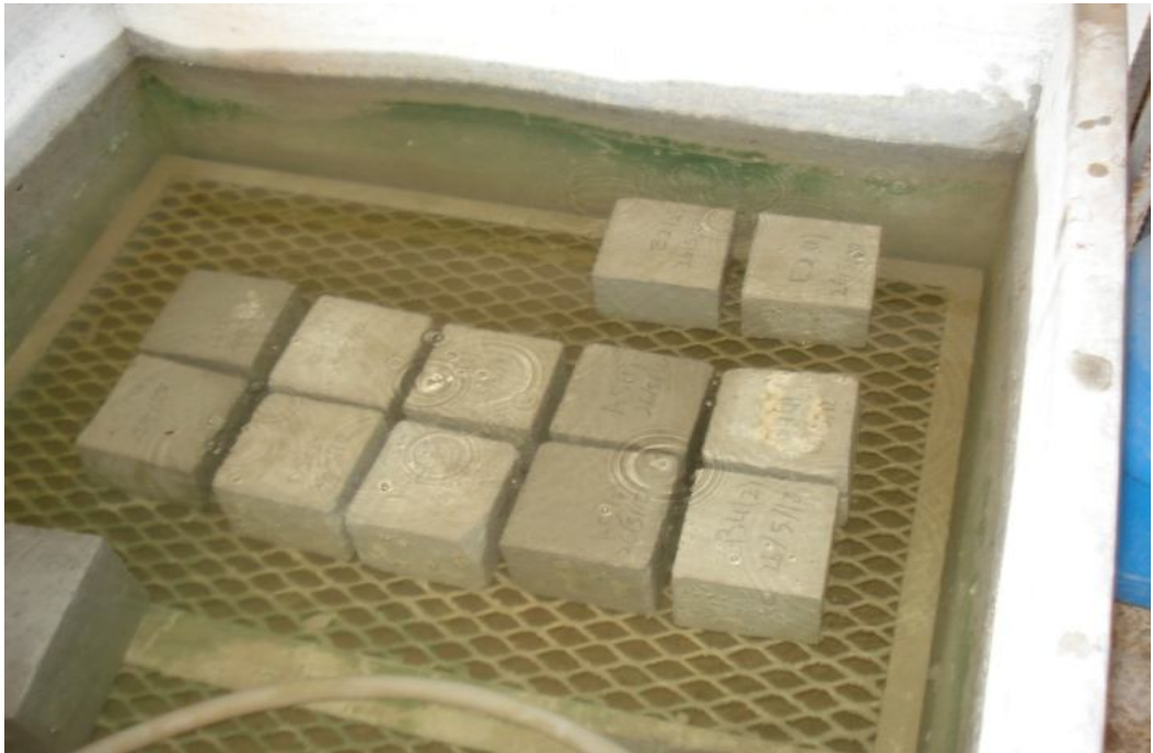
Photo 3.18: Samples were Immersed in Water for 7 days.
