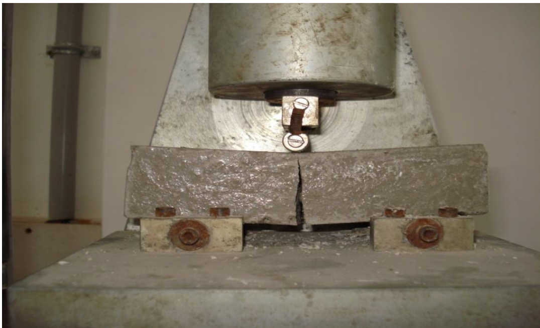
Photo 3.26 : Fracture of Sample in Flexural Test.
