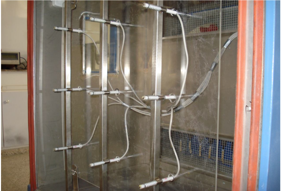
Photo 3.42: Thermo-Couples to Measure the Surface Temperature of Wall Specimen.
