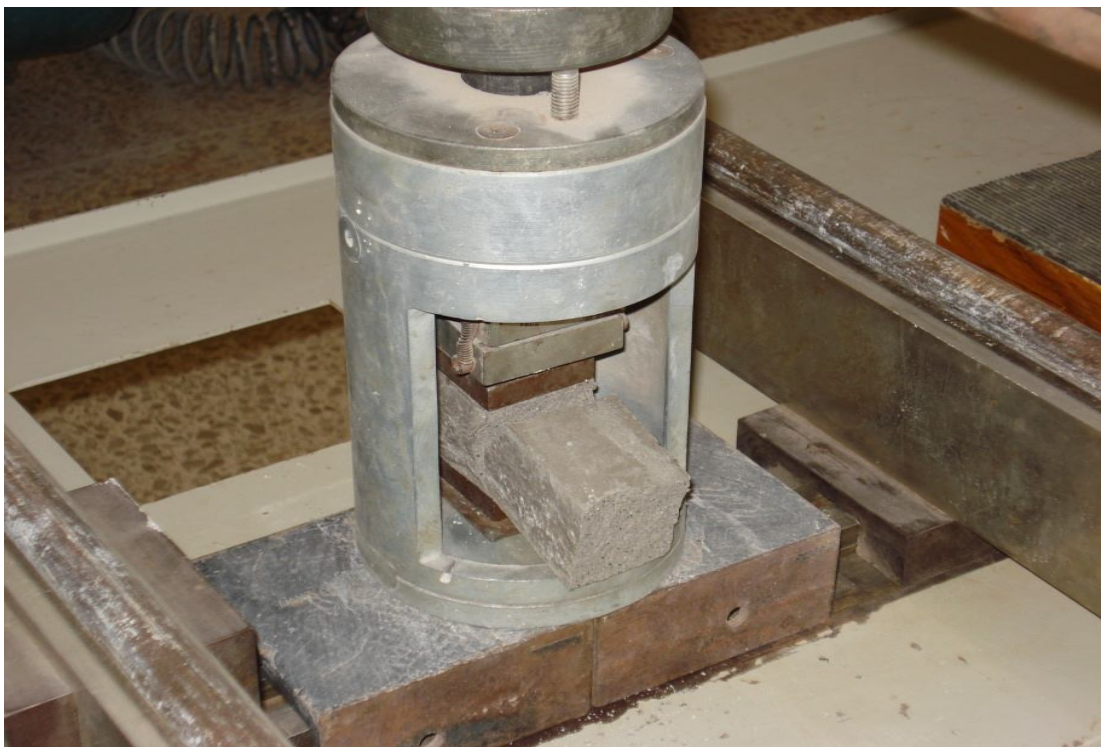
Photo 3.28 : Fracture of Test Specimen Under Compressive Loading.
