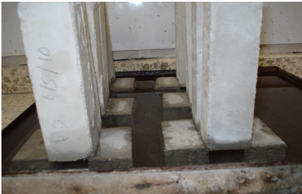
Photo 3.21 : Test Mechanism for Determination of Capillary Water Absorption of Mortar.
