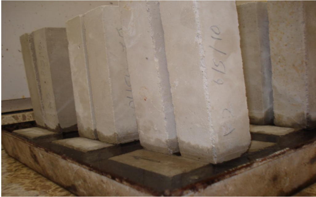
Photo 3.20 : Samples Placed into Water for Testing Capillary Water Absorption of Mortar.
