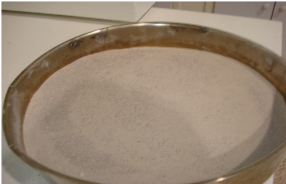
Photo 3.4: Sieved Pumice Aggregates (size \leq 2\text{ mm} )
