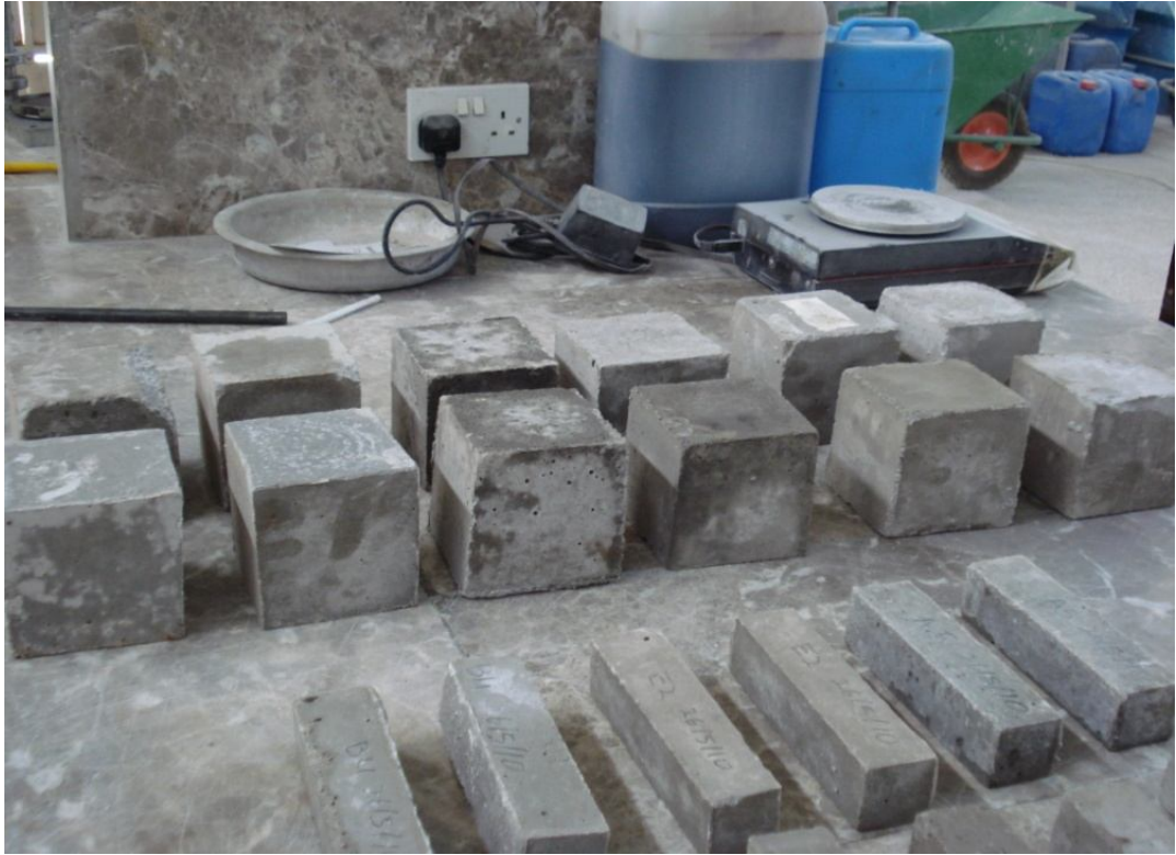
Photo 3.29: Test Specimens (100x100x100 mm) for Pulse Velocity Test
