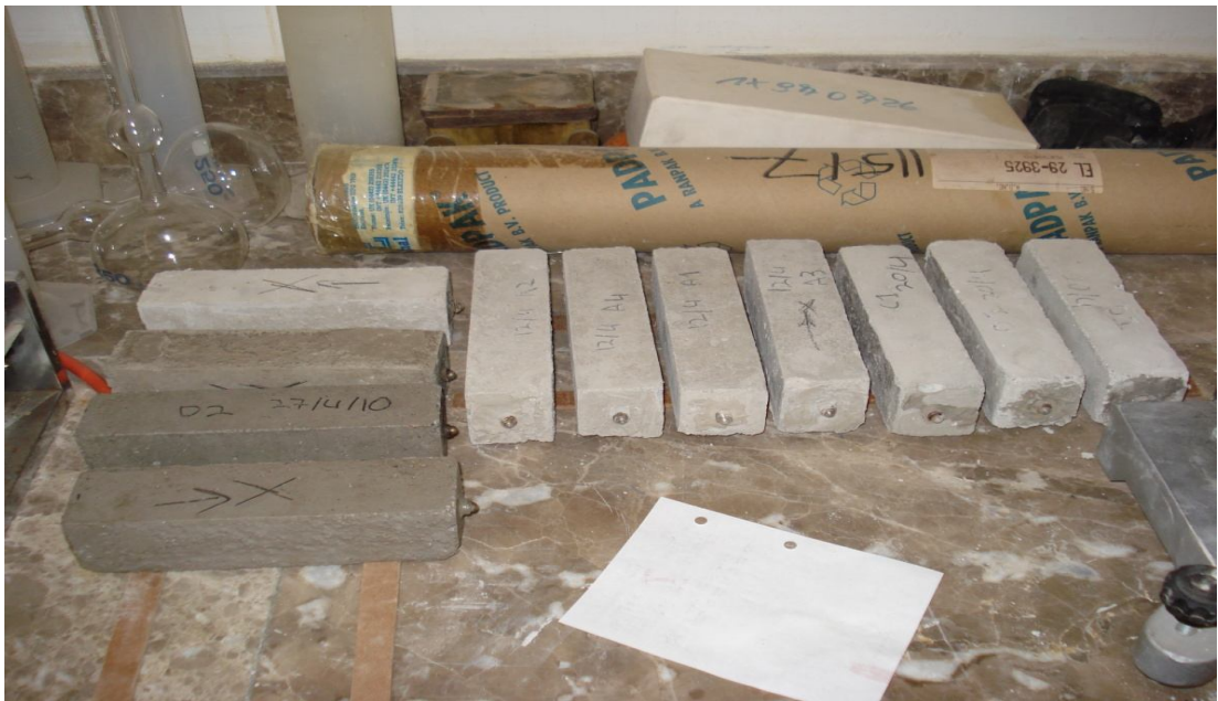
Photo 3.23 : Test Specimes are Located in Air Storage Room for 25 Days.
