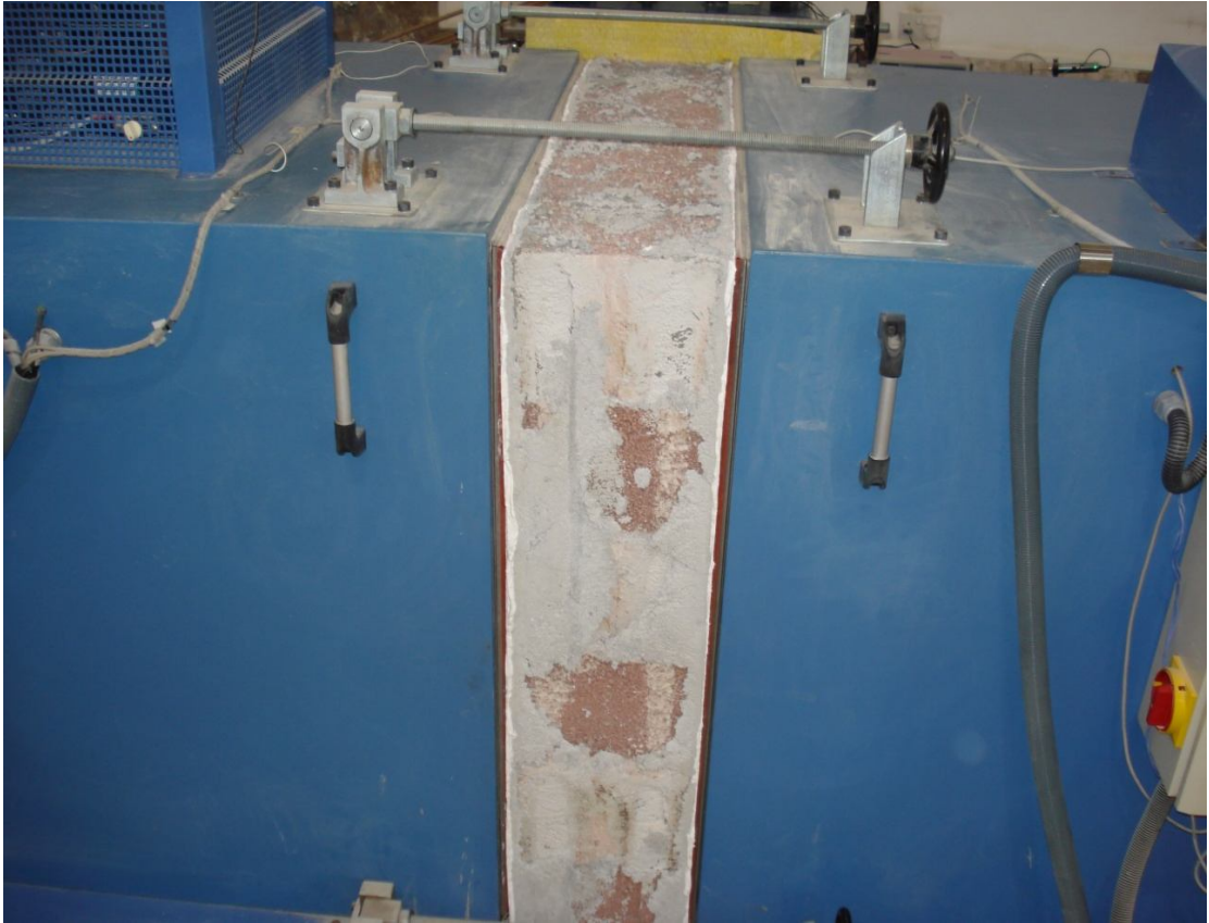
Photo 3.46: Wall Specimen Placed Tightly Between Hot Chamber and Cold Chamber.
