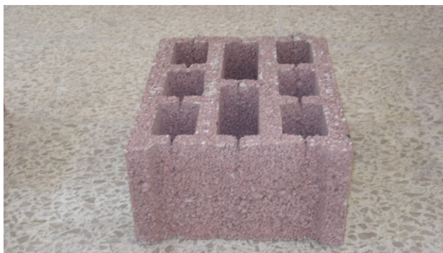
Photo 3.8: Type 3 Pumice block with Dimensions 250 x 390 x 185 mm
