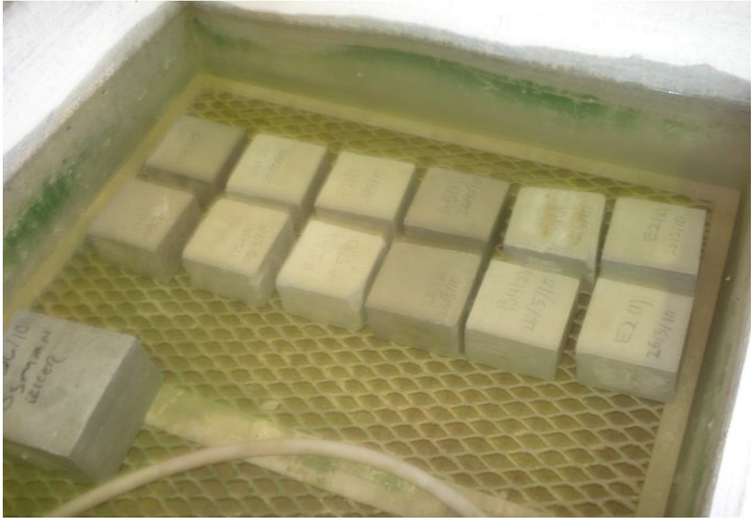
Photo 3.15: Samples for Determination of Hardened Unit Weight of Mortars.
