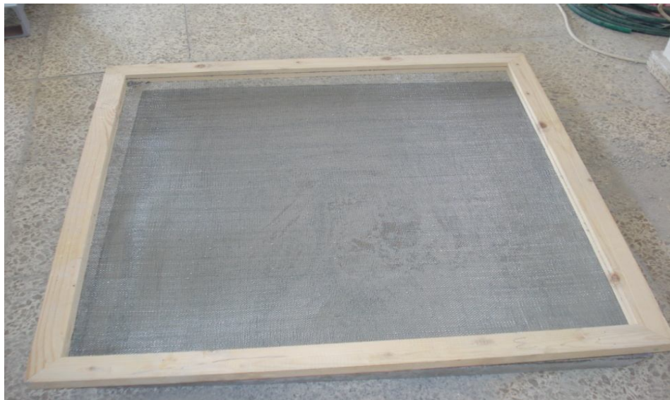
Photo 3.2: Sieve Used to Obtain Required Size of Aggregates.
