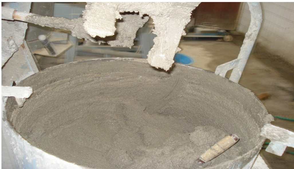
Photo 3.31: Mortar Produced by Large Mixer
