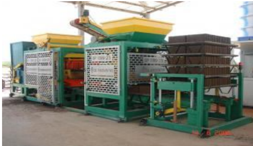
Photo 2.4: Pumice-Block Production Machine
