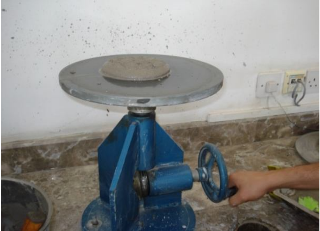
Photo 3.10: Determination of Consistency of Fresh Mortar by Using Flow Table.
