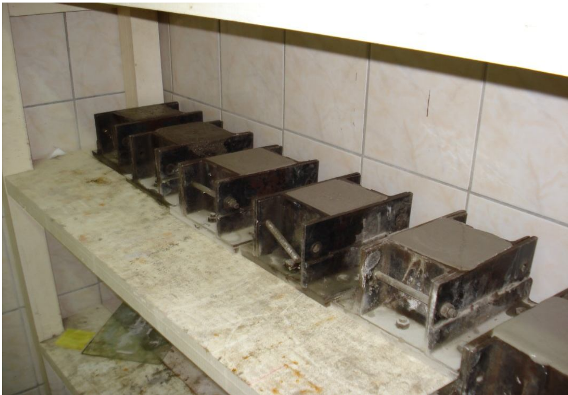
Photo 3.14 : Samples for Testing Fresh Unit Weight of Mortars
