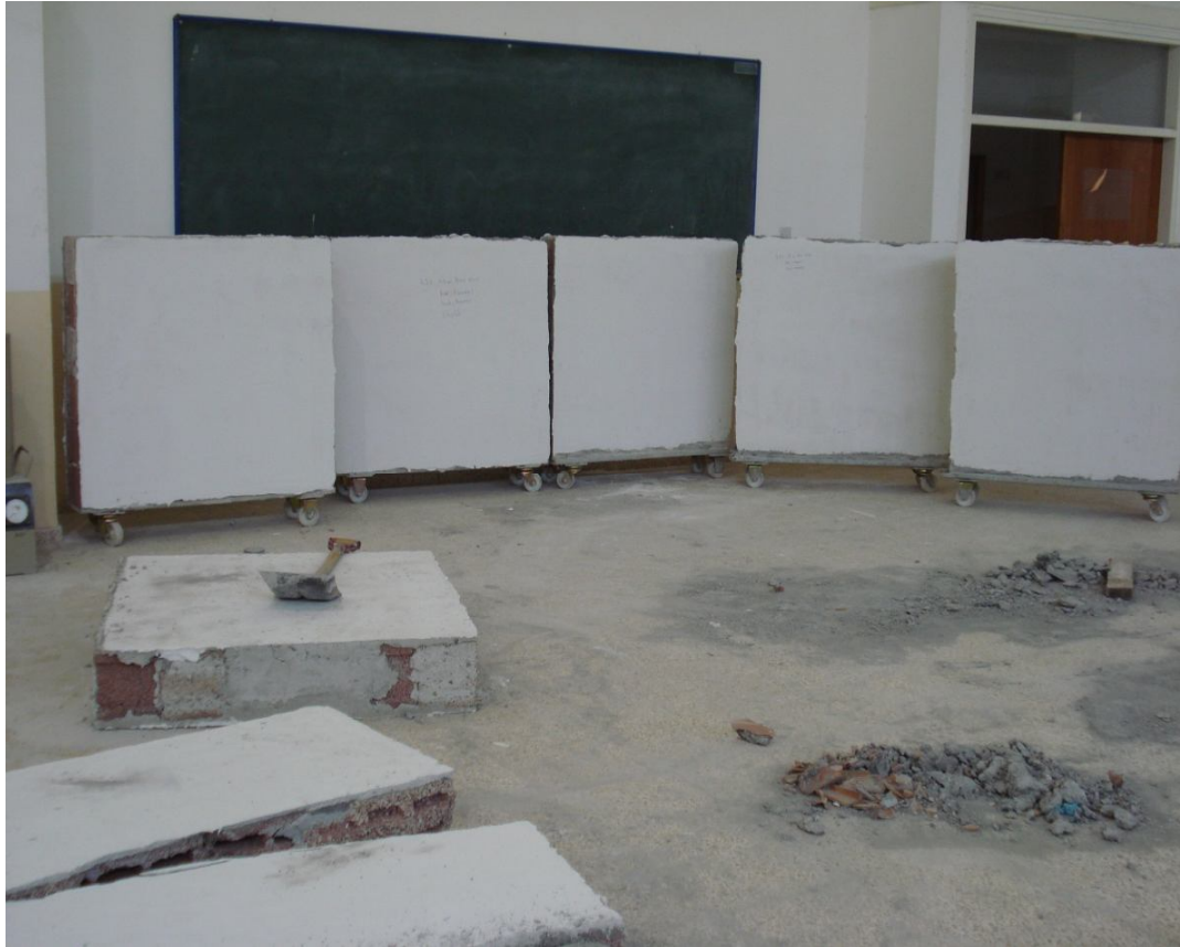
Photo 3.40: Wall Specimens are Ready for Thermal Conductivity Coefficient Test.
