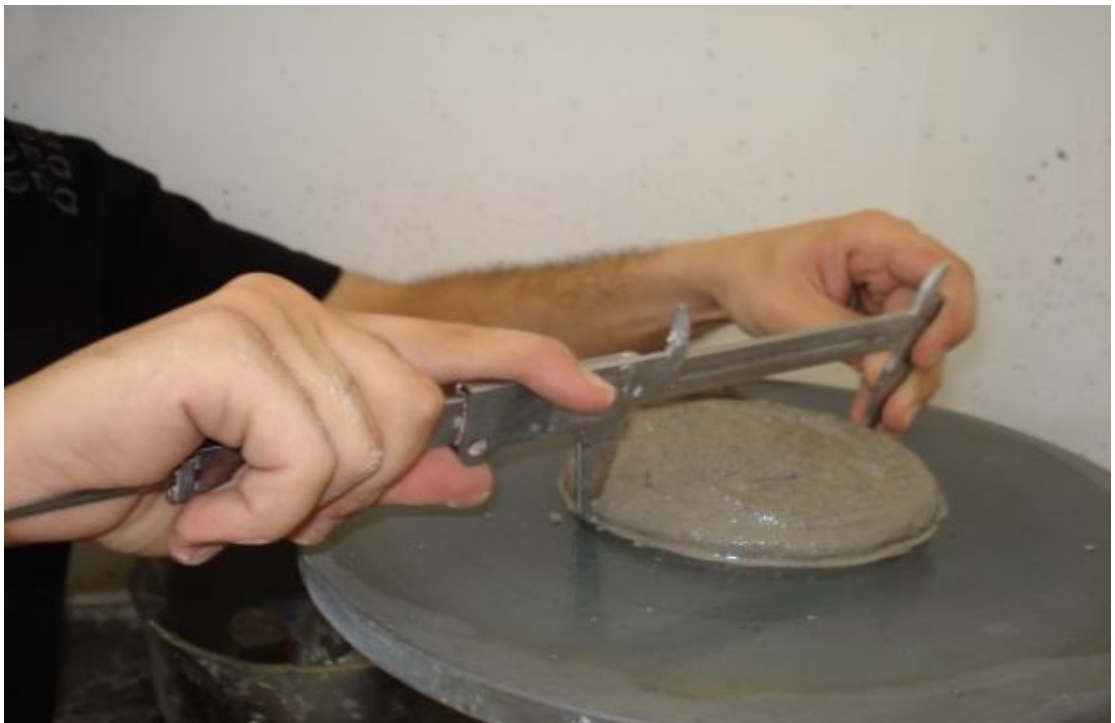
Photo 3.11: Flow Diameter of Fresh Mortar is Measured by Compass.
