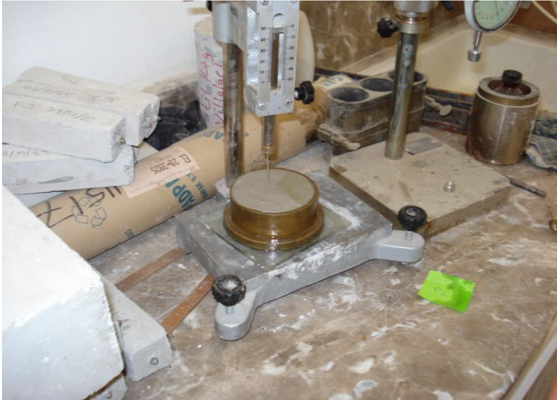
Photo 3.12: Test for Setting Time of Fresh Mortars
