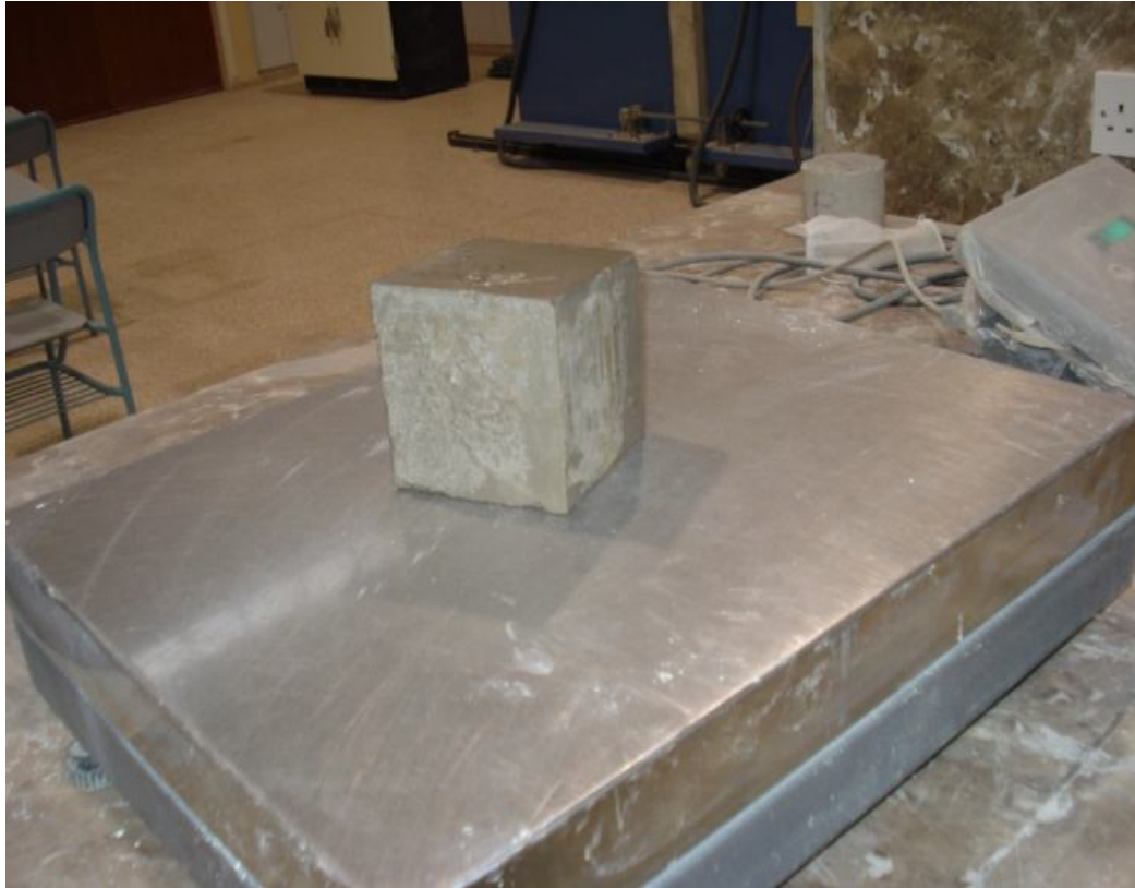
Photo 3.19: Saturated Weight of Samples were Measured.
