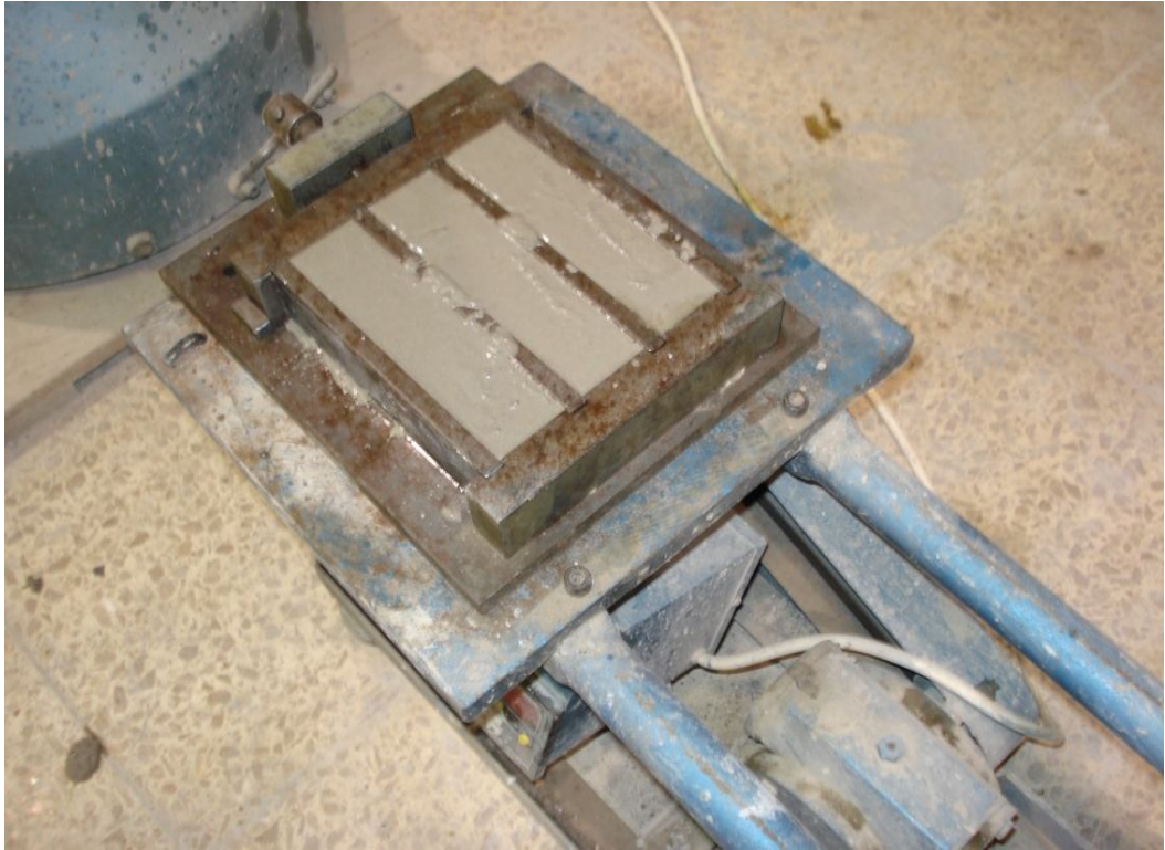
Photo 3.24 : Mortar Samples were Compacted by Jolting Table
