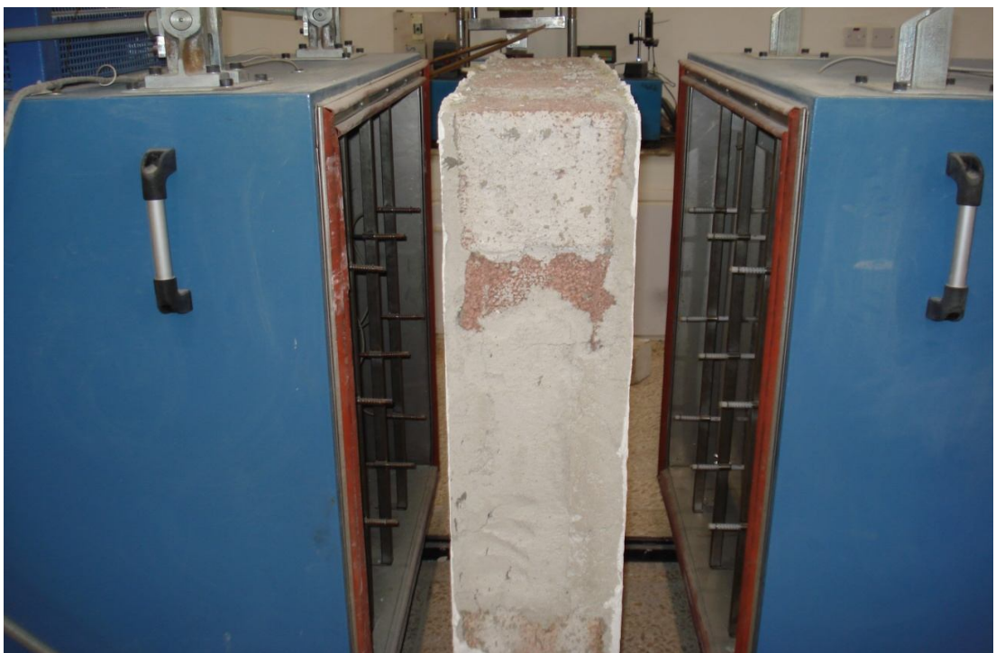
Photo 3.45: Wall Specimen is Placed on Hot-Box Device.
