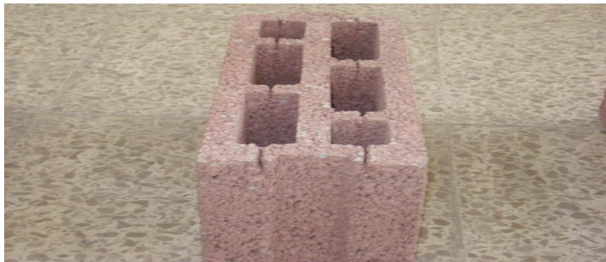
Photo3.6: Type 1 Pumice Block with Dimensions 150 x 390 x 190 mm
