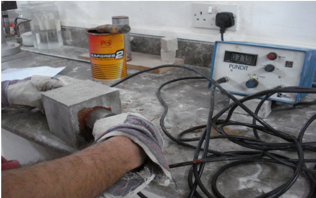
Photo 3.30: Pulse Velocity Test Performed on Mortar Sample.
