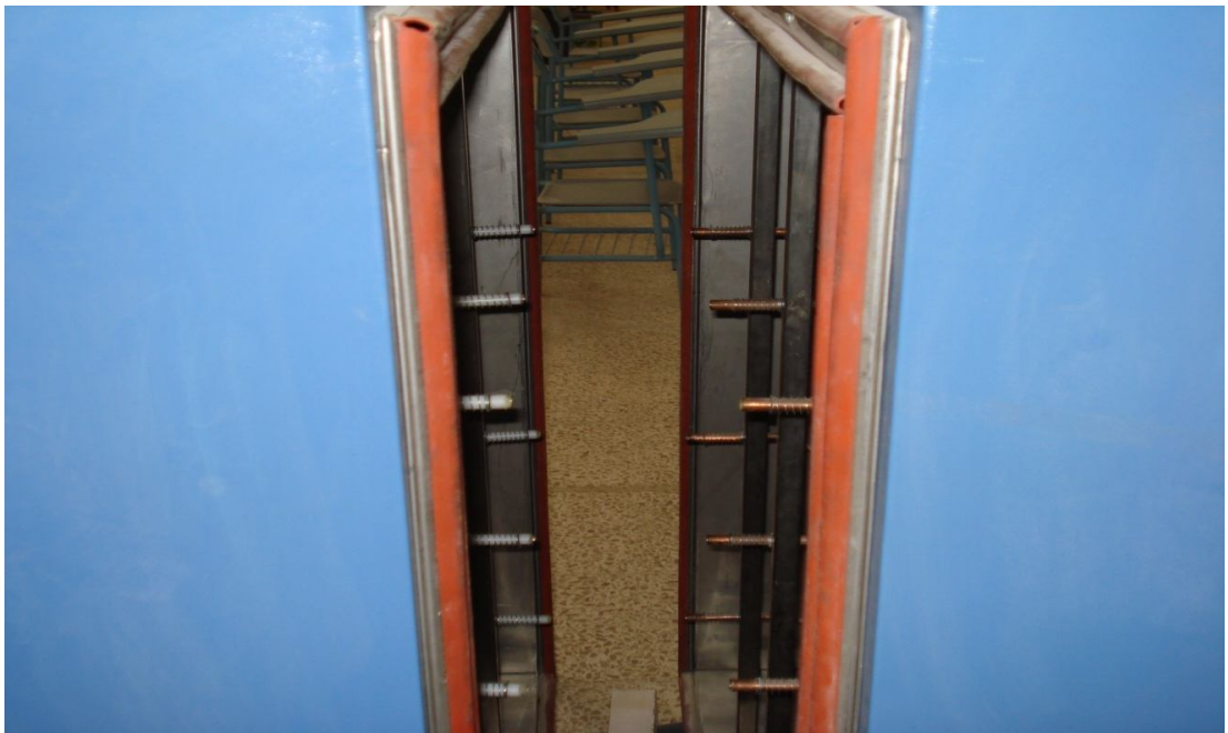
Photo 3.43: Wall Specimen Placed Between Hot (Left Side) and Cold (Right Side) Chambers.
