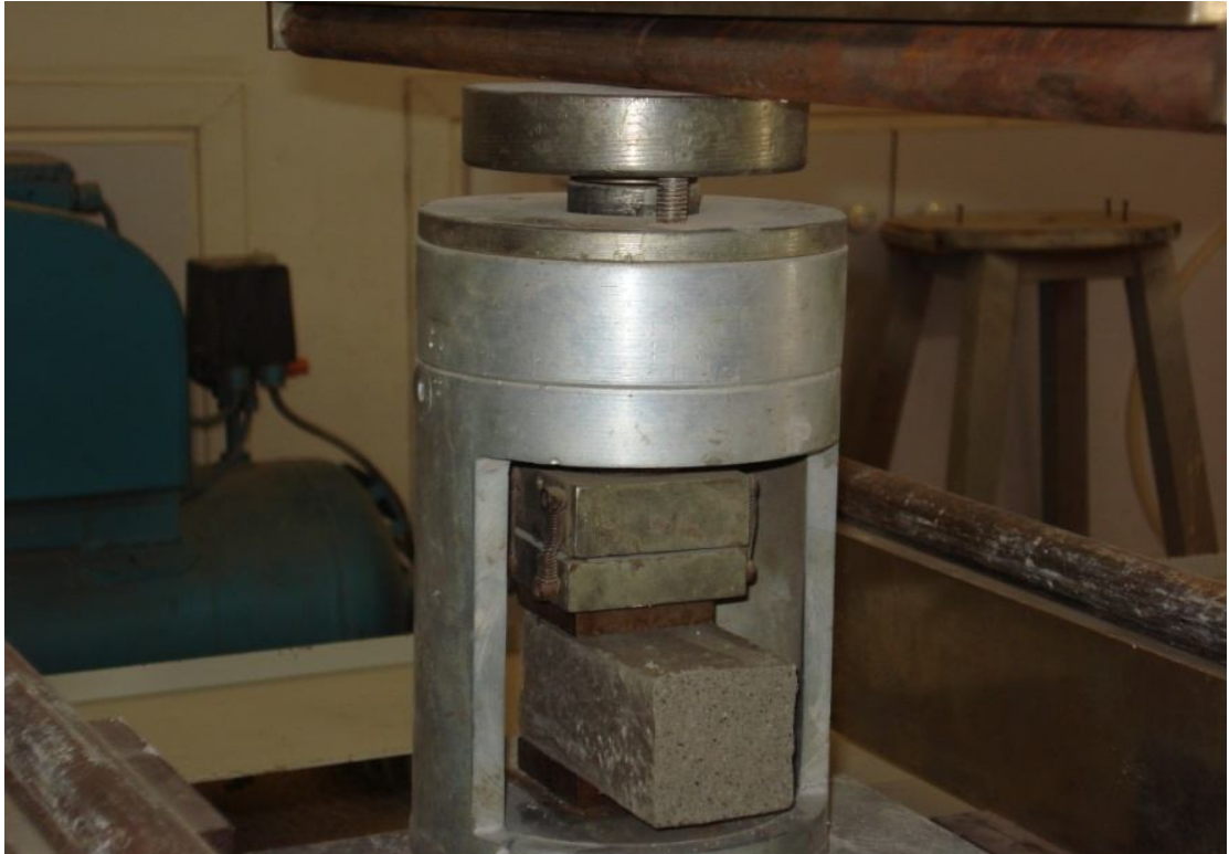
Photo 3.27 : Sample in Compressive Strength Test Machine.
