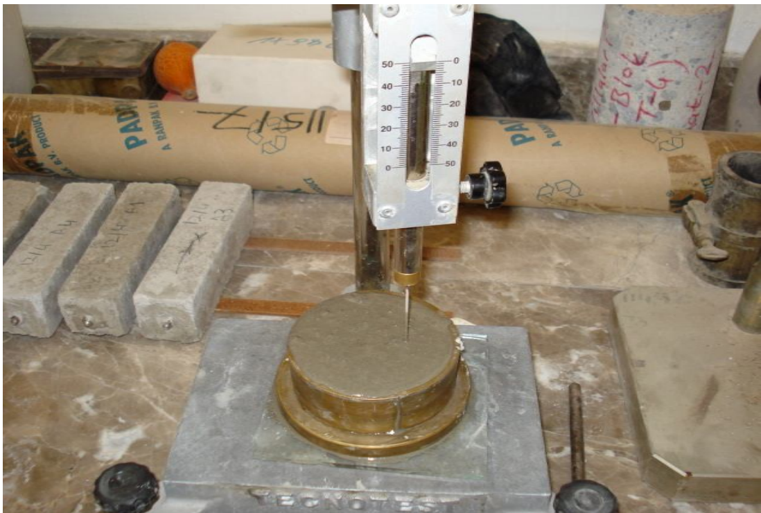
Photo 3.13: Setting Time of Mortar is Determined by Vicat Apparatus.
