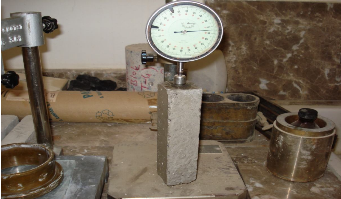
Photo 3.22: Length of Test Specimen is Measured by Length Comparator Apparatus
