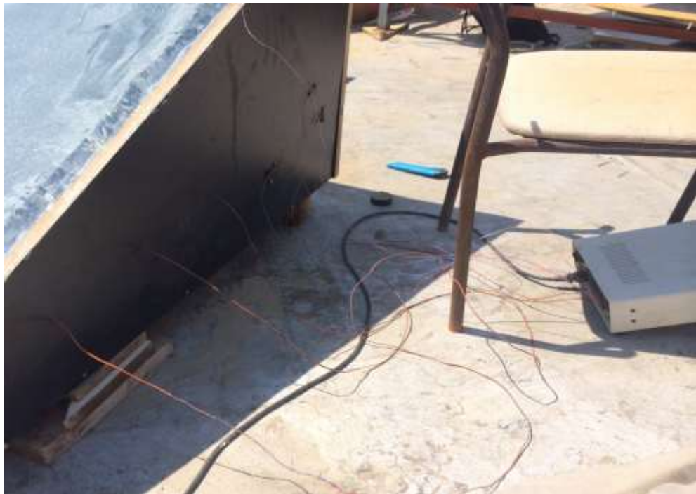
Figure 4.7. View of the connection of digital thermometer and thermocouples.
