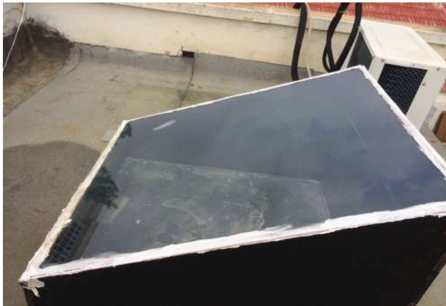
Figure 3.2. A simple conventional solar still.
