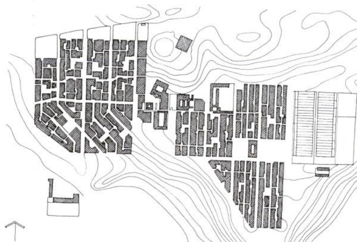
Figure 4.2: Shading of narrow north-south passages
