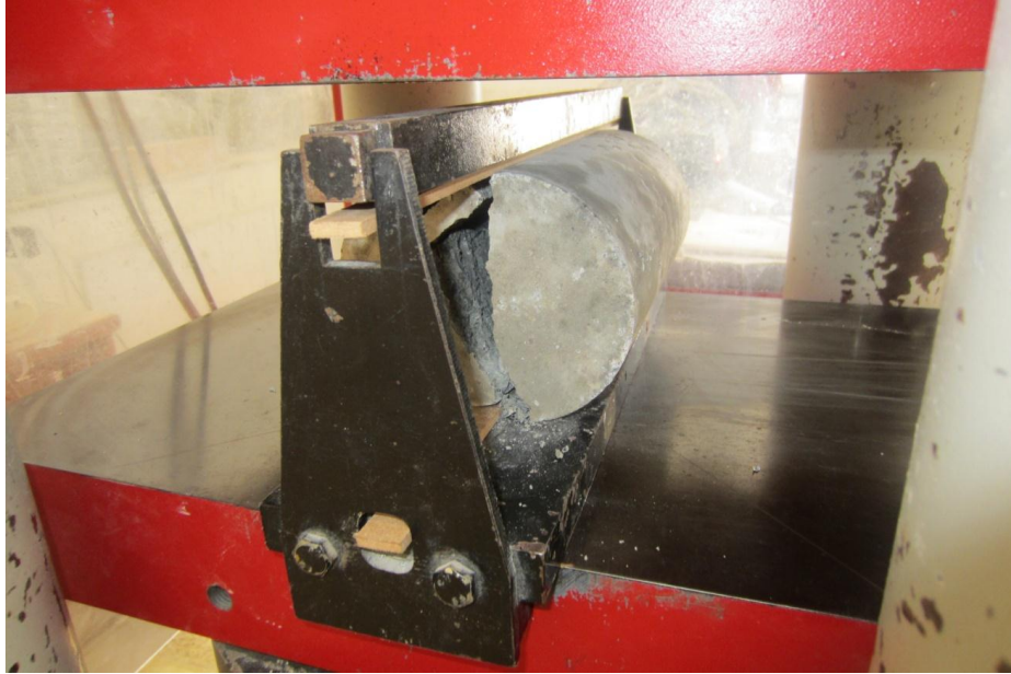
Figure 7: Cylinder specimen failed under splitting tensile test
