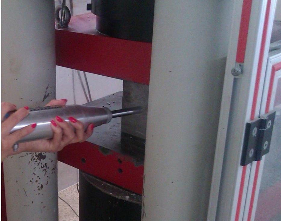
Figure 9: Rebound hammer test on cubic sample
