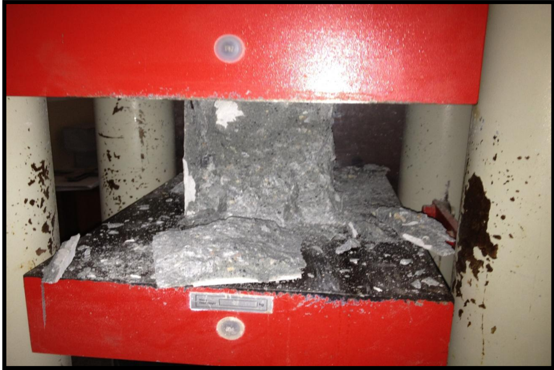
Photo 9 : Crushed specimen after compression test
