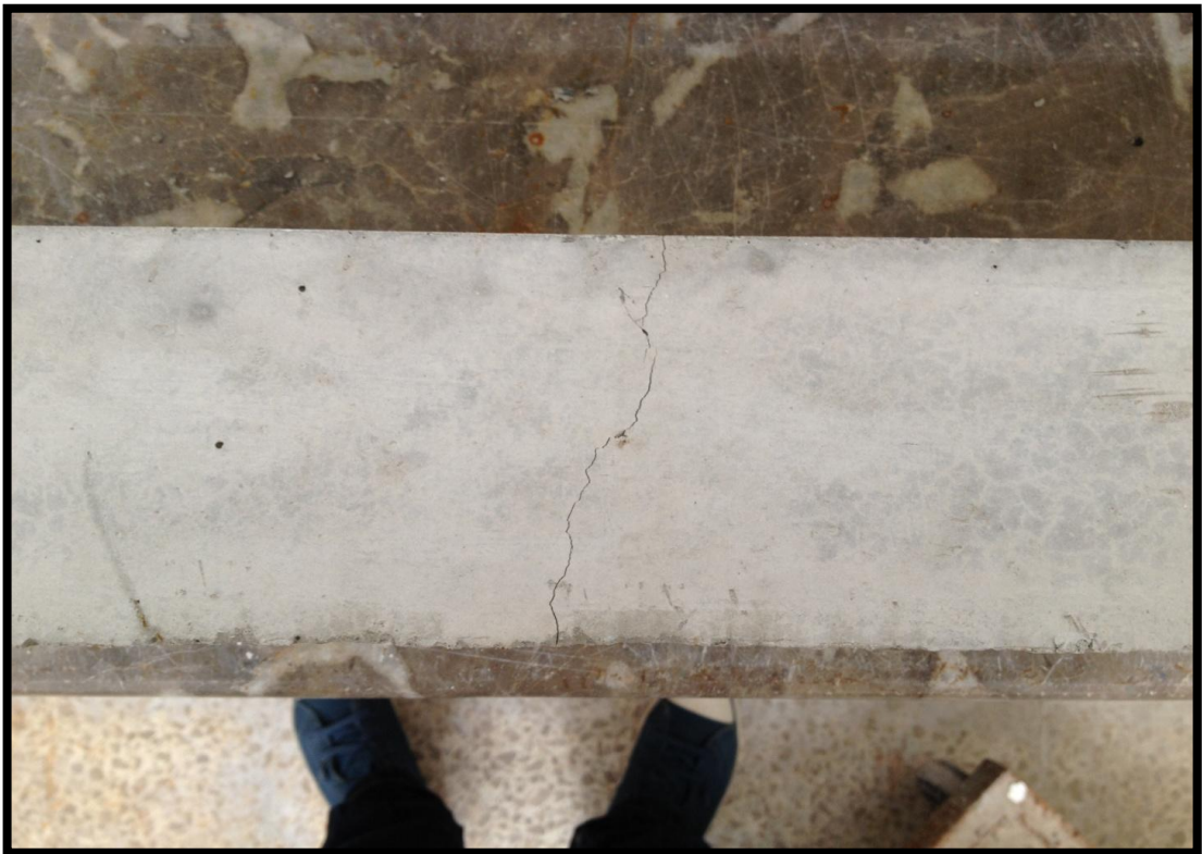
Photo 11: Crack in flexural test beam
