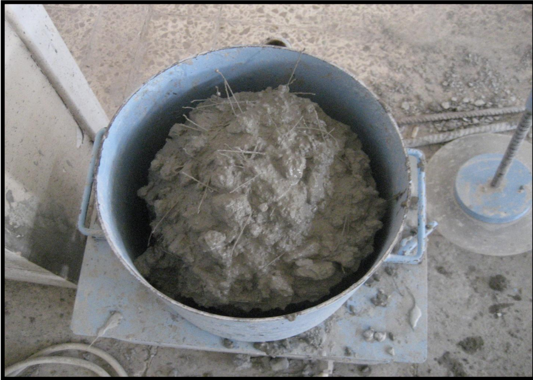
Photo 7: Fresh SFRC in VeBe test pan
