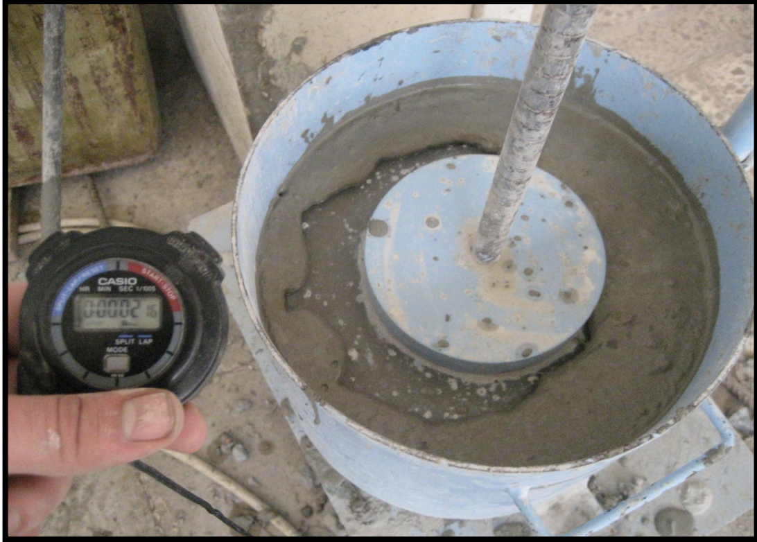
Photo 8: VeBe test completed
