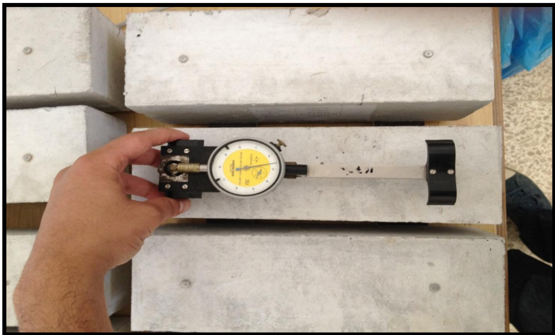
Photo 14: Shrinkage comparator reading
