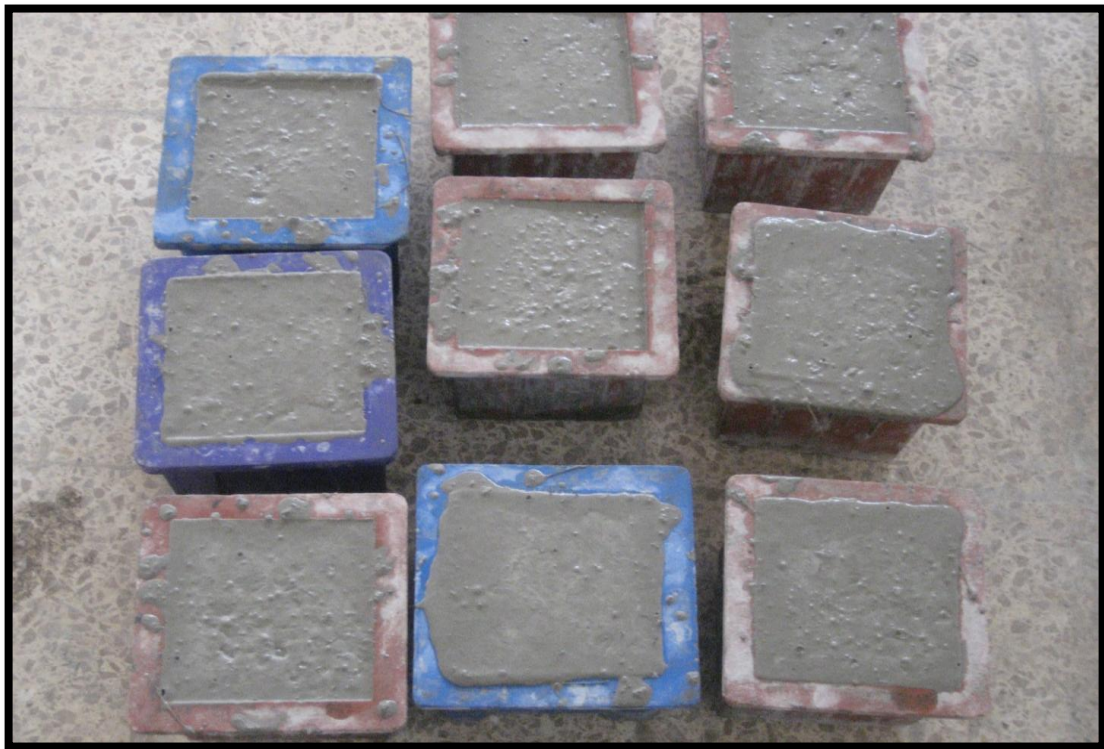
Photo 3: The compressive strength test samples
