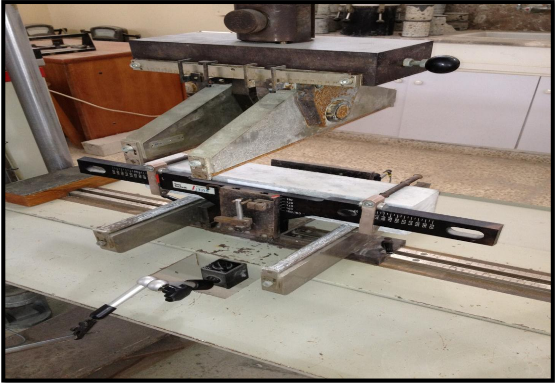
Photo 10: Flexural test apparatus
