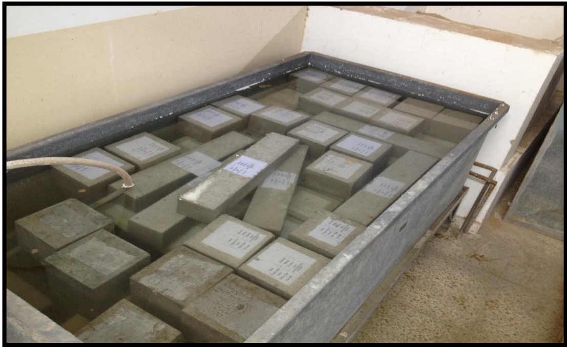
Photo 6: Curing of the specimens in water tank
