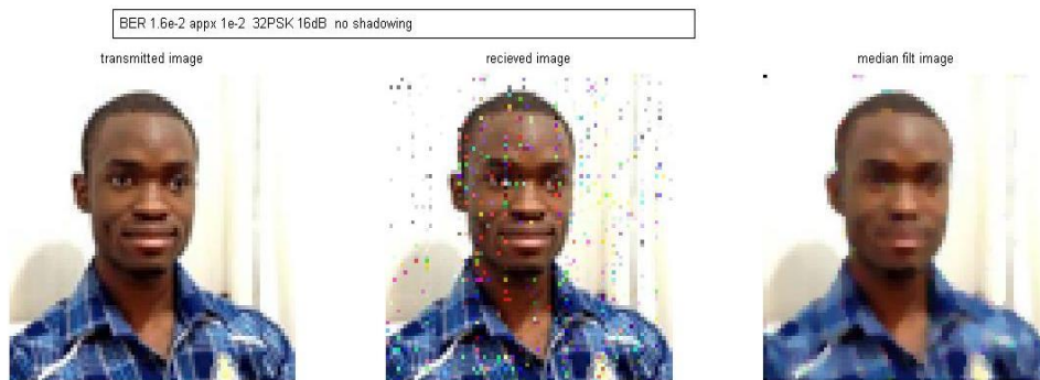
Figure 5.3: Transmitted and Received picture at 10^{-2} and Median filtered received image.
