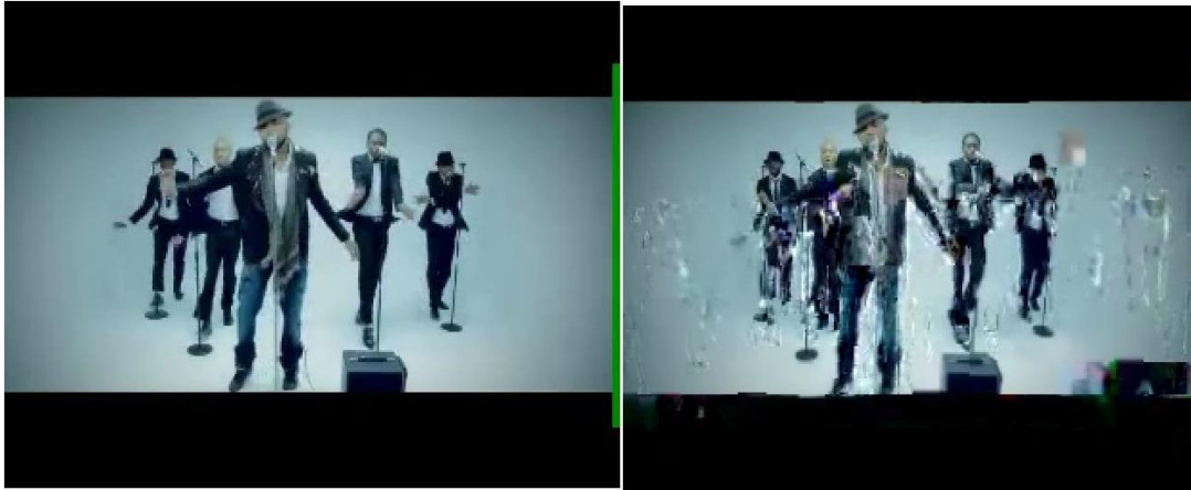
Figure 5.5: A frame of a transmitted and received video over the channel BER 3.95e-5
