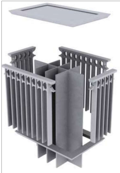
Figure 2.7: 3D model of the duct of the wind catcher. (Mahmoudi Zarandi, 2009)
