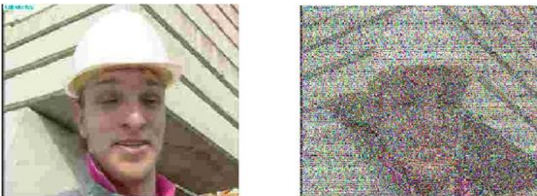
Figure 5.9: 64QAM with scalability (a) original base layer (b) received base layer at SNR=0 dB with BER= 3.1263 \times 10^{-1}
