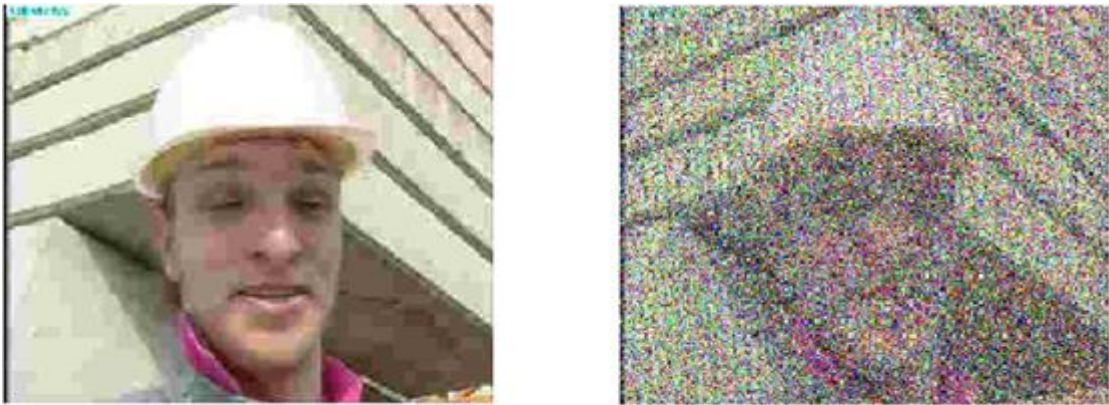
Figure 5.8: 16QAM with scalability (a) original base layer (b) received base layer at SNR=0 dB with BER= 2.3405 \times 10^{-1}
