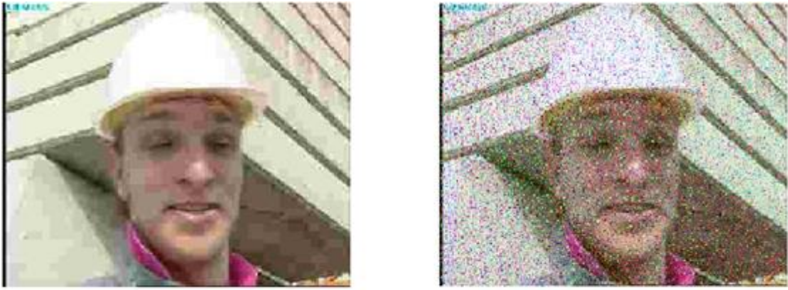
Figure 5.7: QPSK with scalability (a) original base layer (b) received base layer at SNR=0 dB with BER= 6.9994 \times 10^{-2}
