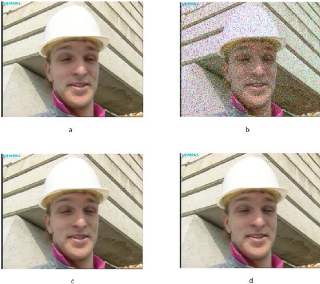
Figure 5.4: QPSK without scalability (a) original (b) received at SNR=0 dB with BER= 6.9888 \times 10^{-2} (c) received at SNR=13 dB with BER= 2.1773 \times 10^{-5} (d) received at SNR=20 dB with BER= 6.5729 \times 10^{-6}
