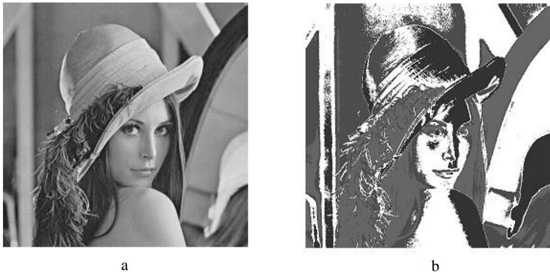
Figure 2.15: a) 256×256 Lena gray scale image b) segmented image using FCM clustering with ( c=4 )
