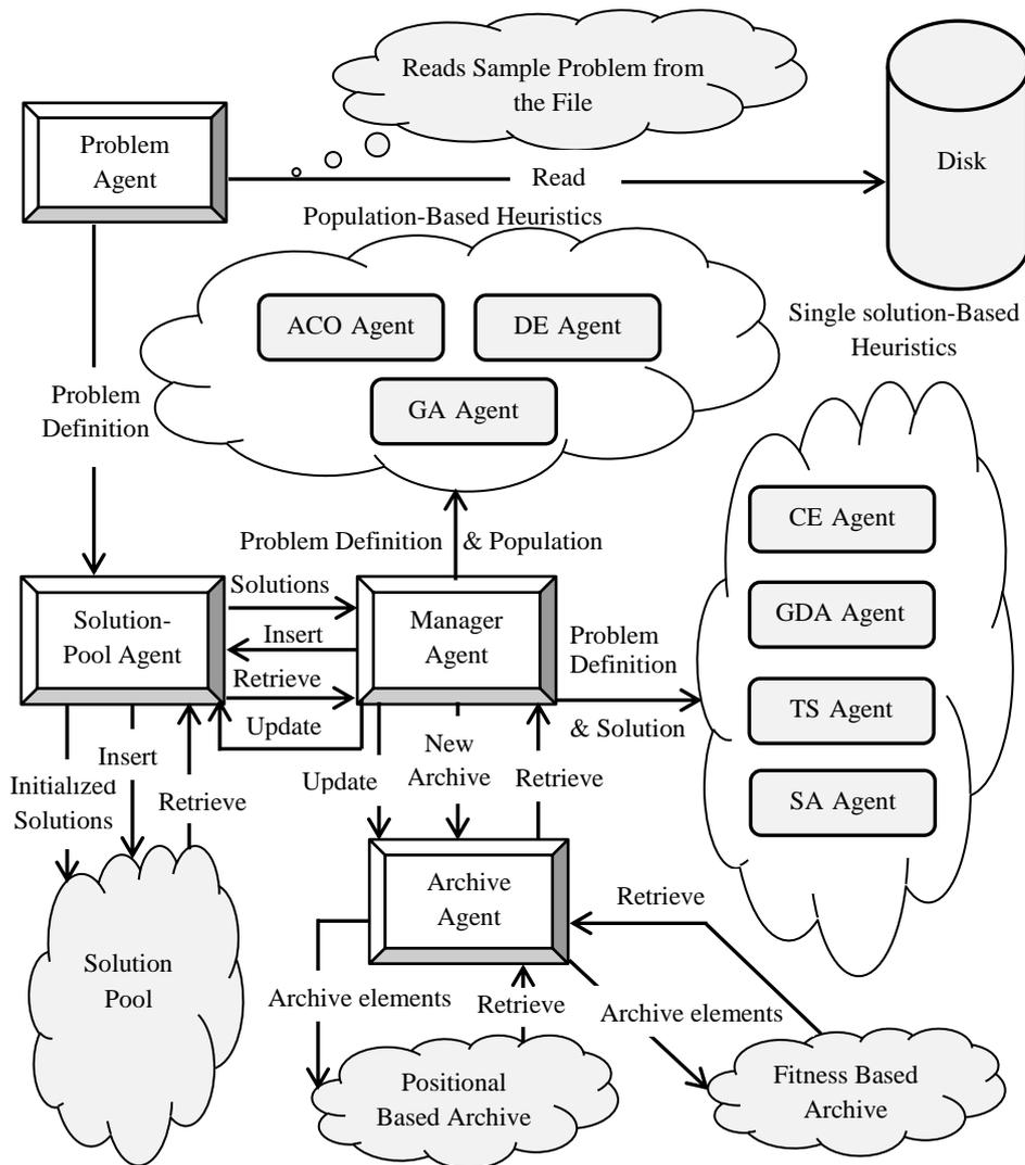
Figure 4.1. Architectural description of LBMAS concerning its metaheuristic agents and the four functional agents
