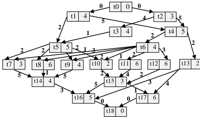
Figure 7.1. A sample task graph representing a particular MSP [16]
