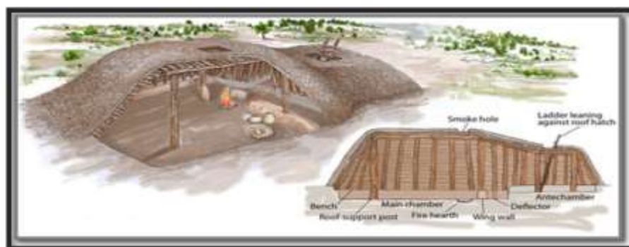
Figure 13: The structure of Pit House in Native American architecture
