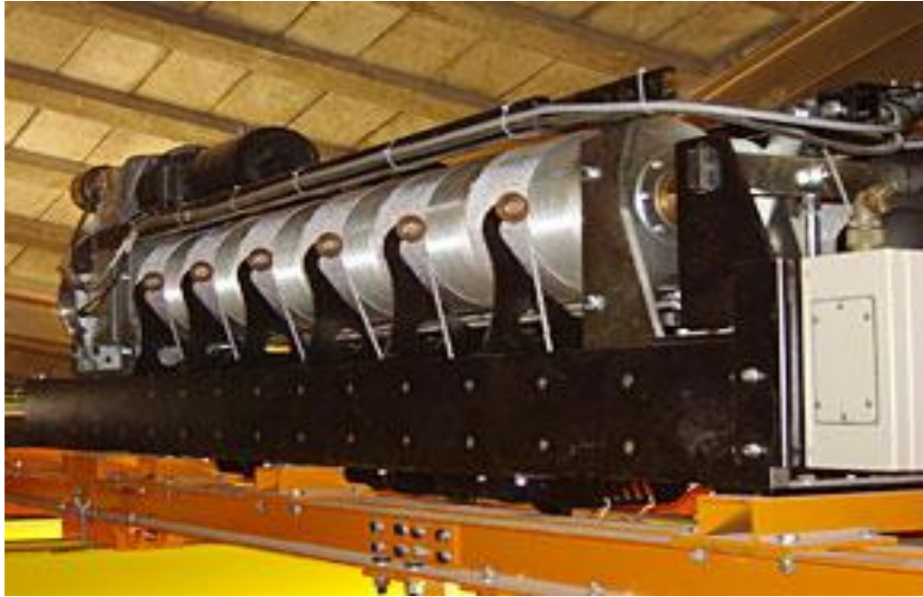
Figure 35: Stage machinery for scene changes example-“One major refurbishment carried out at the Royal Festival Hall over the last few years added to the infrastructure in order to make this process easier and quicker, while adding to the flexibility of the venue” (Bryant, stage_technologies_transforms_royal_festival_hall, 2008)
