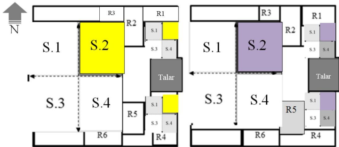
Figure 105: Evaluation of thermal comfort in open and semi-open spaces on the ground floor and first floor of a traditional building in Kashan during the winter and summer
