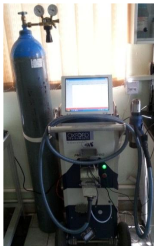
Figure 3.8: PMI-Master pro metal analyzer by Argon gas
