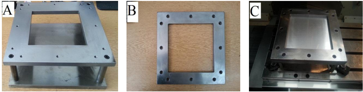
Figure 3.6: (A) Bottom and lower plates, (B) Upper plate, (C) Complete clamping system fixed on machine table
