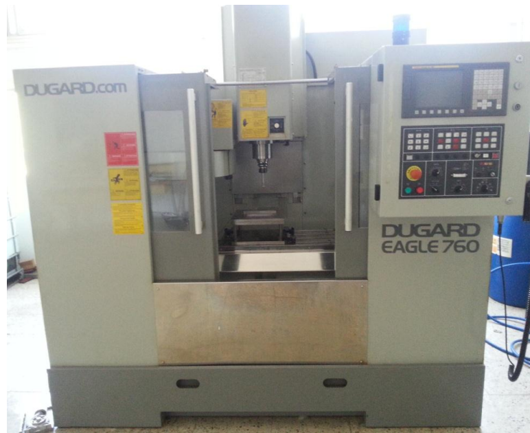
Figure 3.4: Dugard ECO 760 CNC milling Machine
