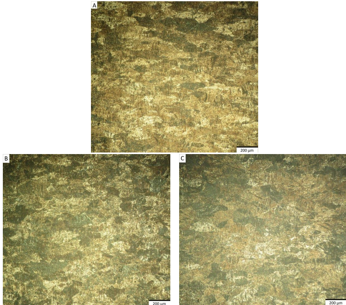
Figure 4.13: Effect of lubrications on AA5754 Aluminium Alloy with 100X magnification, (A) base material, (B) Hydraulic oil, (C) Grease.
