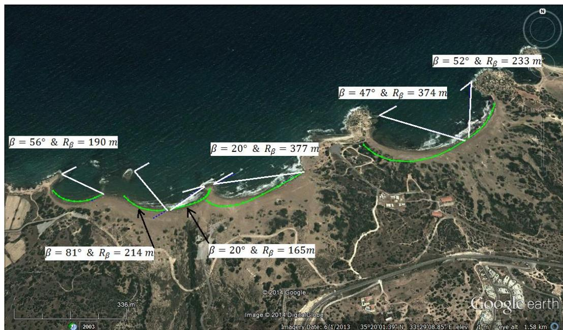
Figure 36. General implementation of the PBSE to different headland bays of the Alagadi Beach, using unsubmerged headland tips as diffraction points
