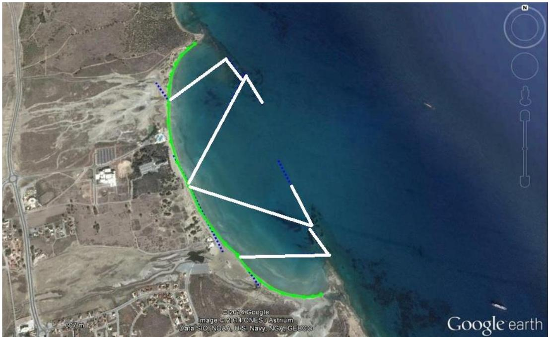
Figure 28. Multiple diffraction point used to fit the shoreline periphery of the beach by MEPBAY
