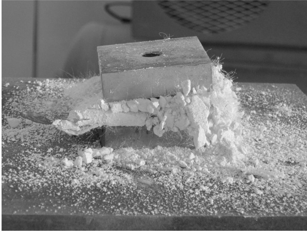
Figure 3.27: Failure of LCMP in Compressive Strength Test
