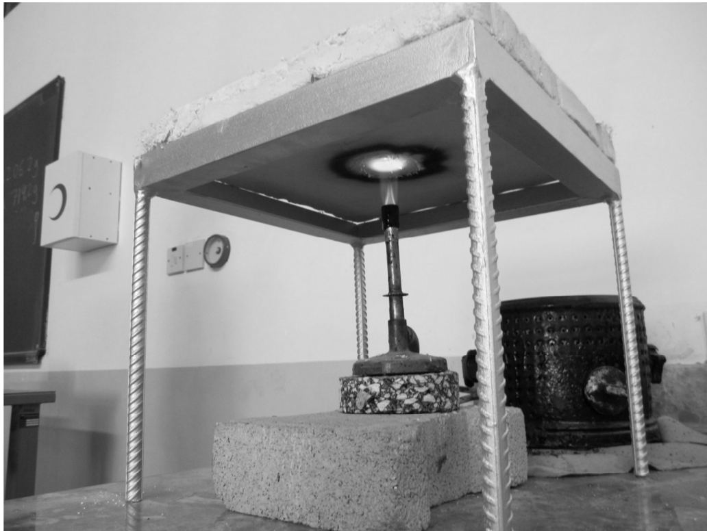
Figure 3.11: Fire Test (ASTM E 84)
