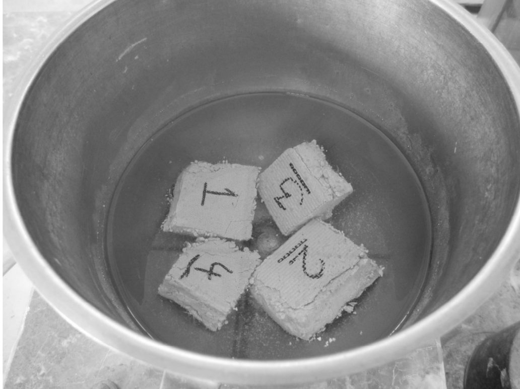
Figure 3.28: LCMP Samples which are Sank in the Water
