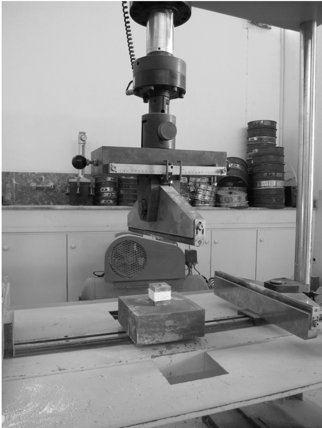
Figure 3.26: Compressive Strength Test on LCMP
