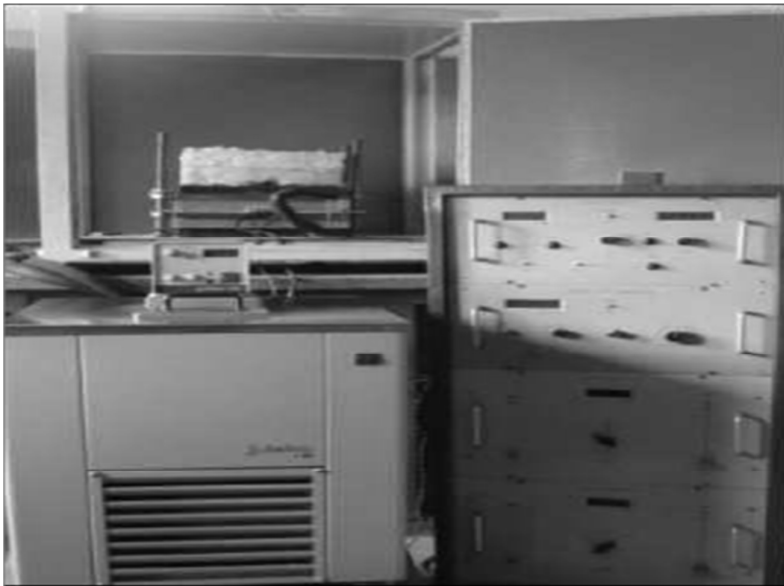
Figure 3.7: Guarded Hot Plate Apparatus
