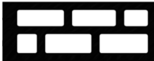
Figure 3.18: Schematic Shape of Clay Brick (300 x 100 x 240 mm)
