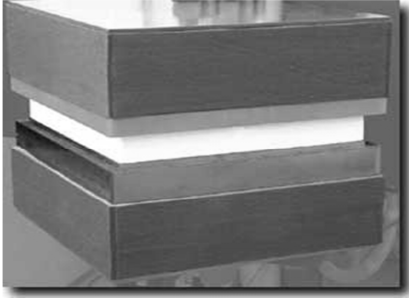
Figure 3.8: Plates of Guarded Hot Plate Apparatus
