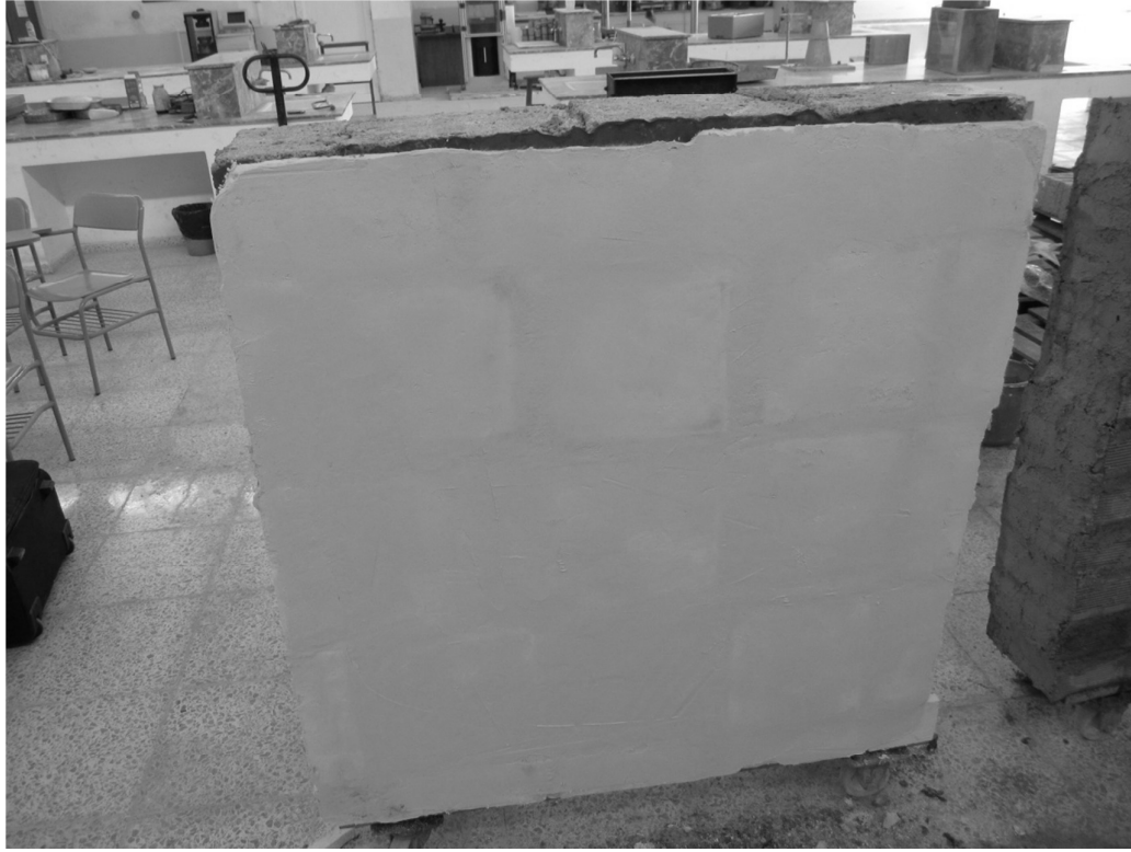
Figure 3.24: Insulated Wall with LCMP
