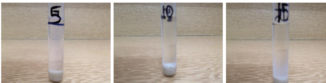
Figure 3.6. Effect of Reaction Time of Copolymerization of Calcium Alginate With BzMA
