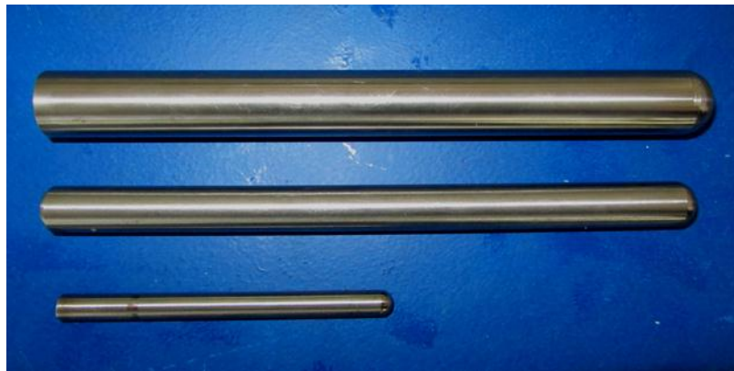
Figure3. 10: Forming tools for SPIF
