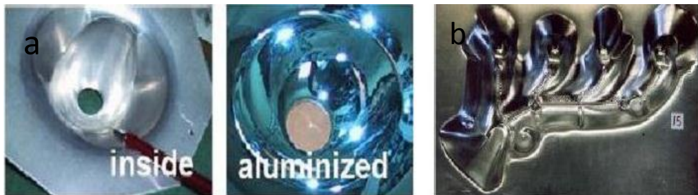
Figure1. 7: a) Reflexive surface for headlights & b) automotive heat/vibration shield
