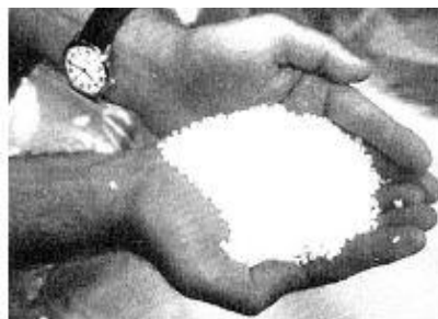
Figure1. 11: Plastic pellets are the raw material in many shaping processes for polymer
