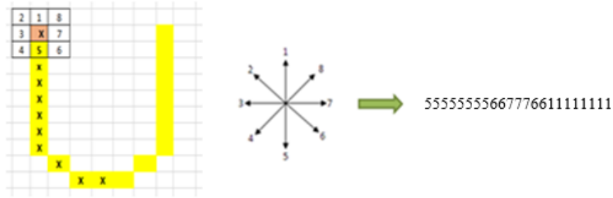
(a) (b) Figure 4.8: Tracing algorithm (a) Character tracing (b) Extracted chain code
