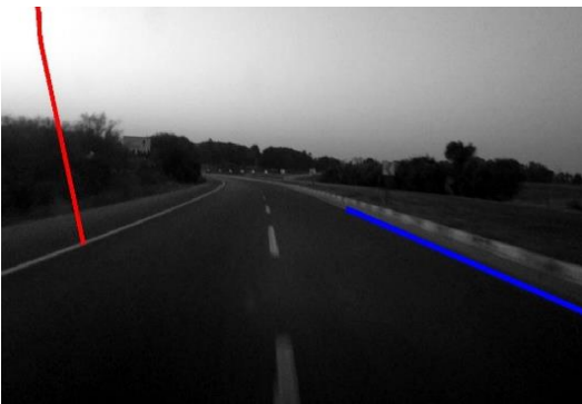
Figure 4.11: Incorrect detections on ROAD-22 custom video.
