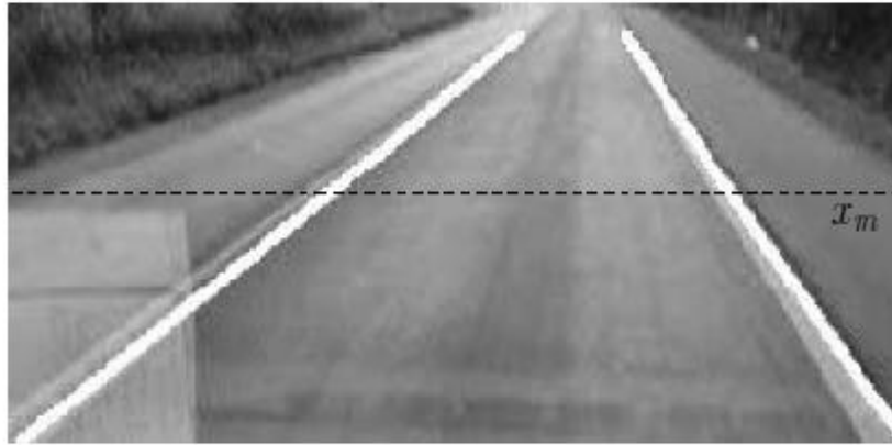
Figure 3.1: The dashed line indicates the border between the near and far fields [7].
