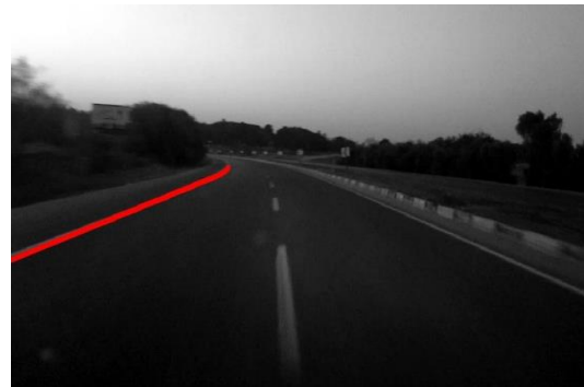
Figure 4.11: Incorrect detections on ROAD-22 custom video.
