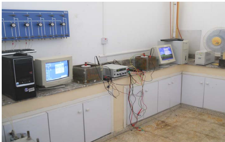
Figure 5.6. Accelerated Corrosion Test Layout
