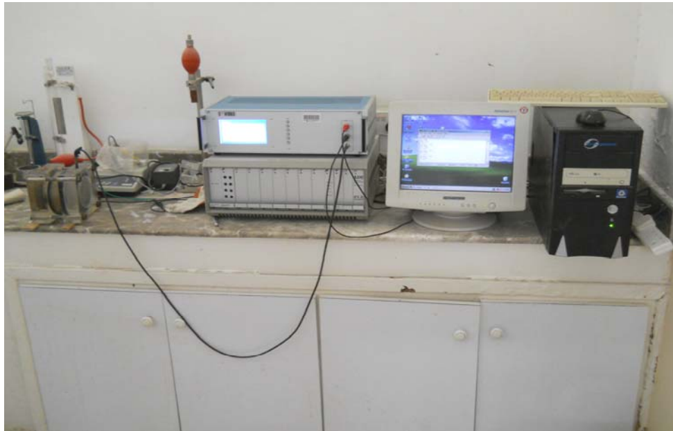
Figure 5.5. Rapid Chloride Permeability Test Assemble
