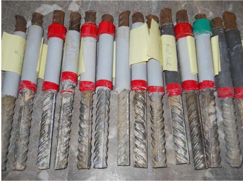
Figure 6.67. Some of the Corrosion Test Reinforcements
