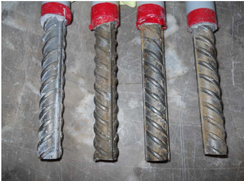
Figure 6.68. Close View of Some Corrosion Test Reinforcements
