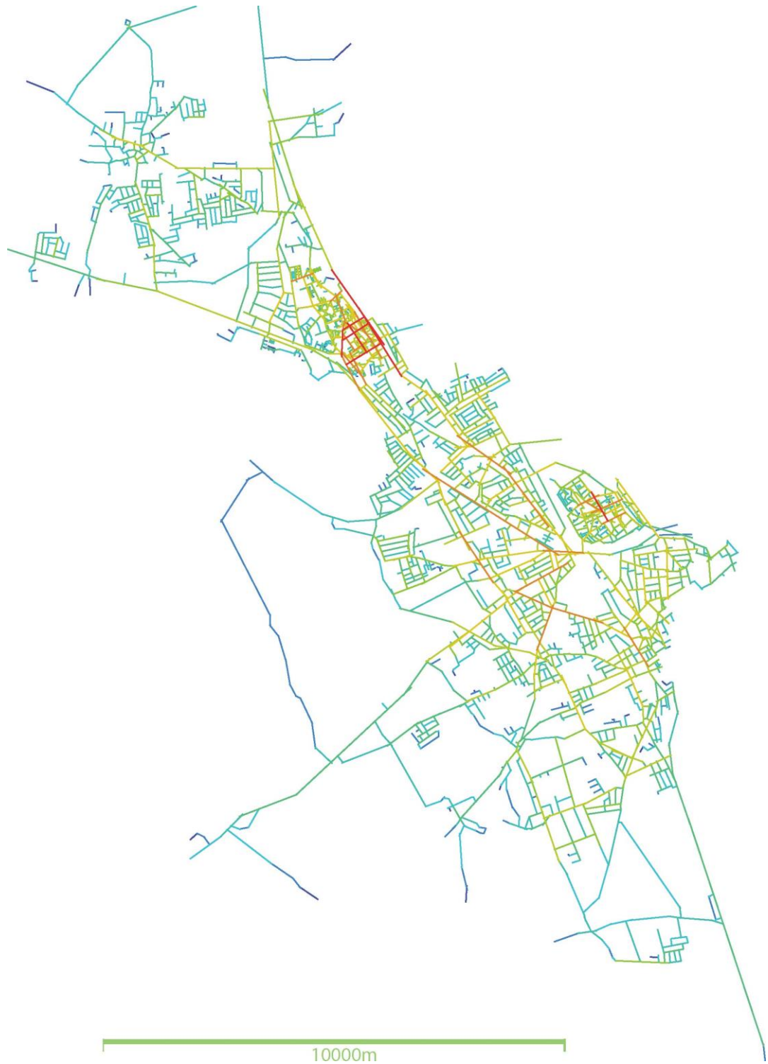
Figure 30. Local integration of Famagusta, the colors represent a spectrum between dark blue as the lowest and red as the highest integration factor, By Author.
