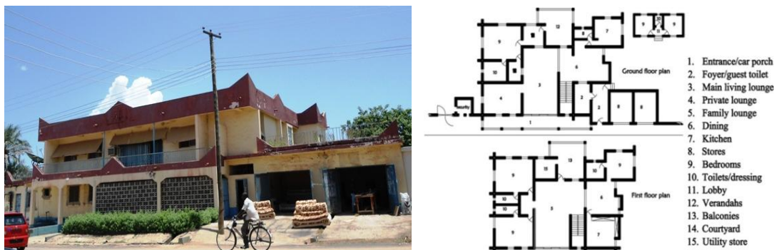
Figure 4.3: Pictorial view and plan of a postmodern residence showing the early revival of traditional pinnacles. Photo by author
