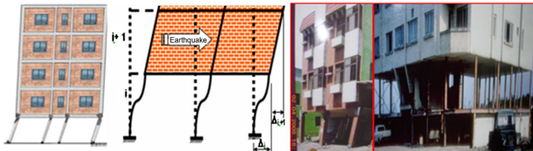
Figure 3.15. Behavior of Soft-Storey During Earthquake (Kirac, Dogan and Ozbasaran 2011)
