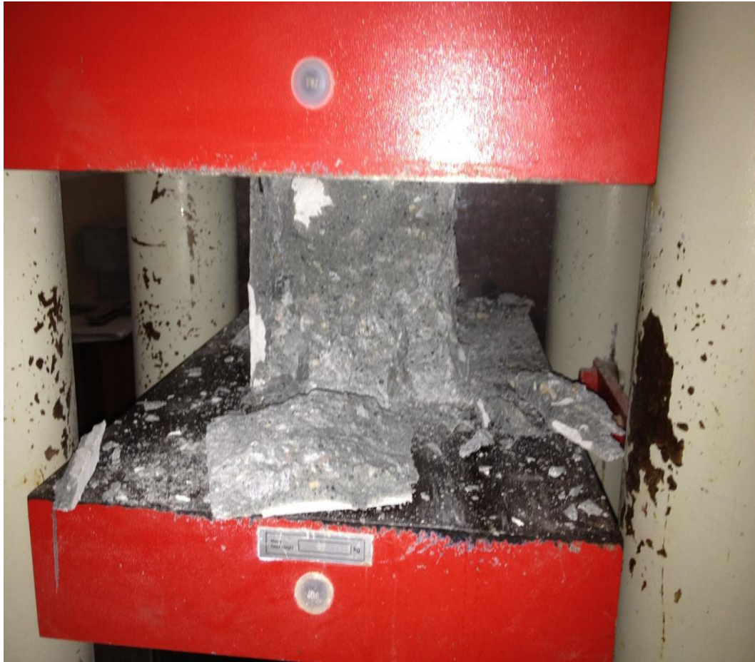
Figure 3.10: Crushed sample under compression load
