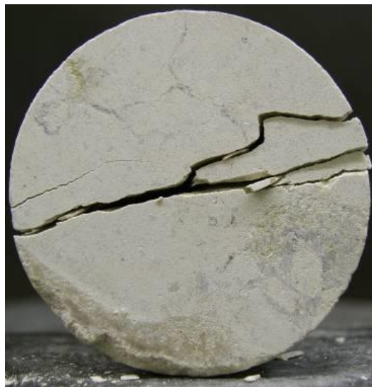
Figure 3.12: Crushed specimen after splitting test
