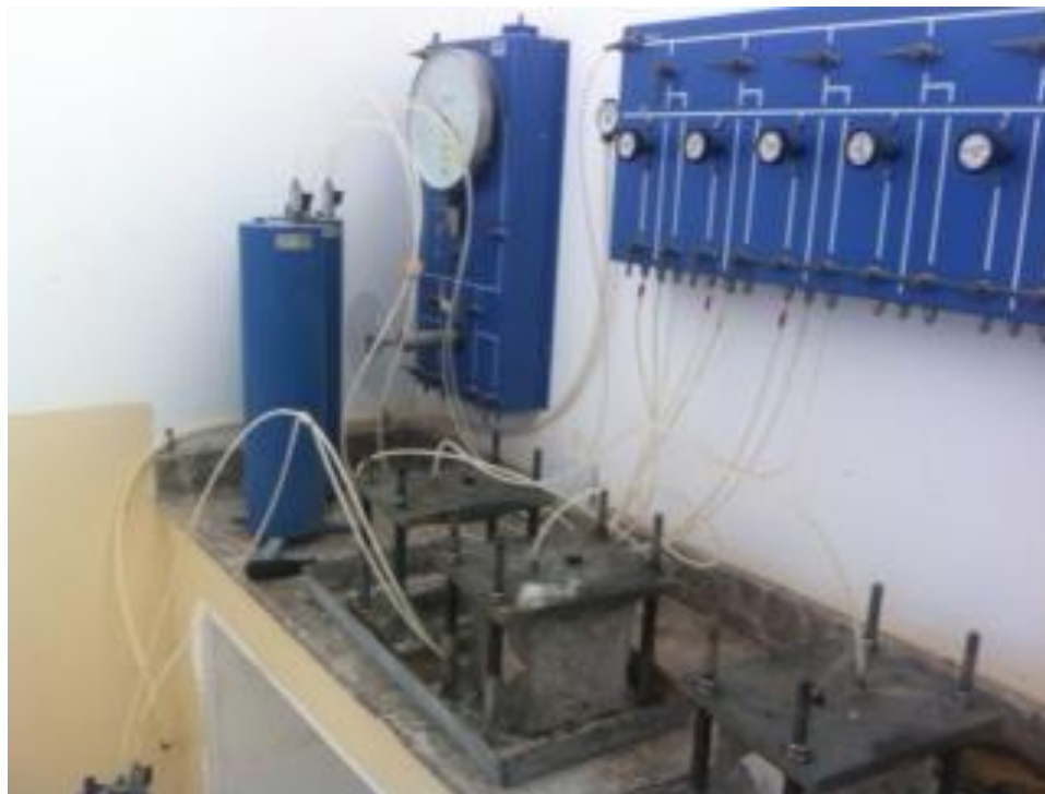
Figure 3.16: Permeability test apparatus
