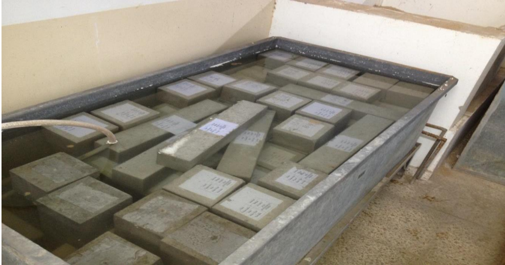
Figure 3.7: Water tank for curing
