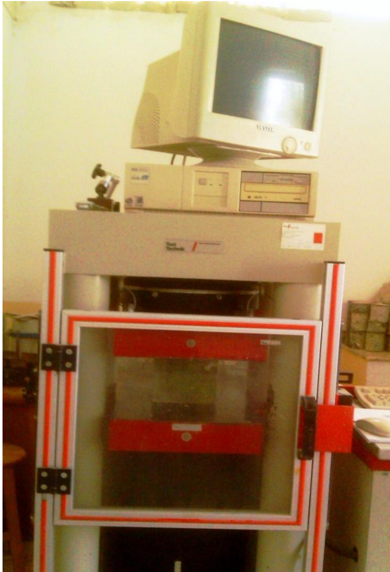
Figure 3.9: Compression test system
