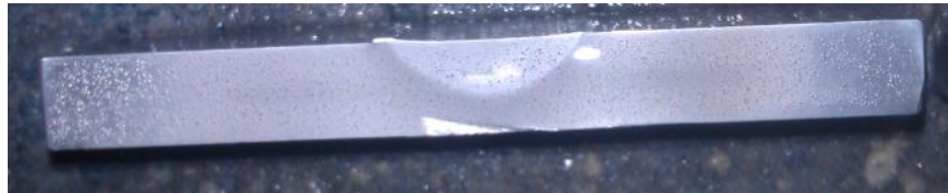
Figure 3.19: Heat Affected Zone (HAZ) After Etching Process
