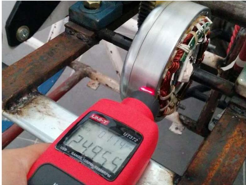
Figure 53: Motor spinning speed measurement setup
