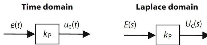
Figure 8: Proportional control term block diagram
