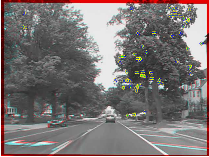
Figure 5.5: Correct Correspondences Based on RANSAC Paradigm
