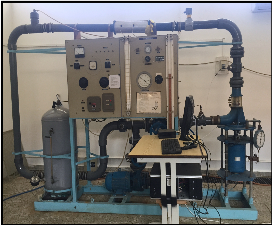
Figure 4.1: Revitalized Axial flow pump/turbine test rig
