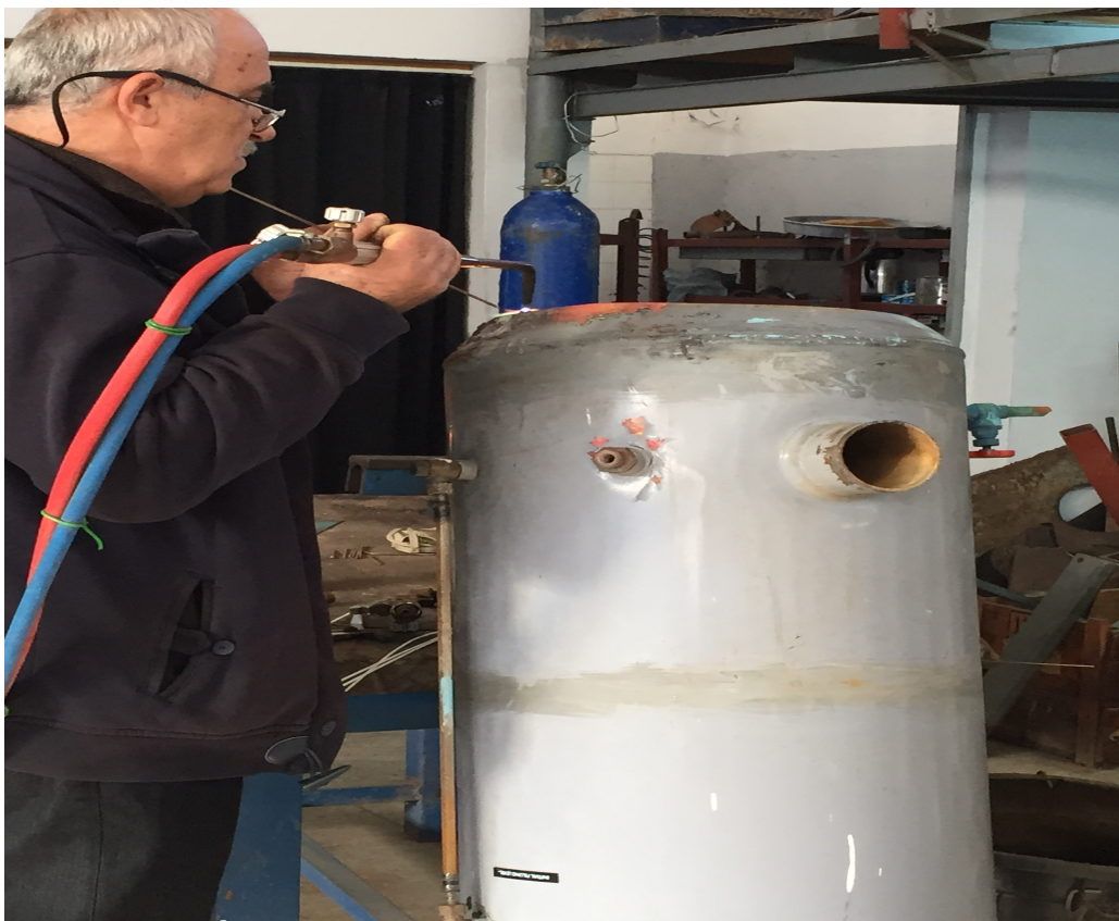
Figure 3.2: Welding the reservoir
