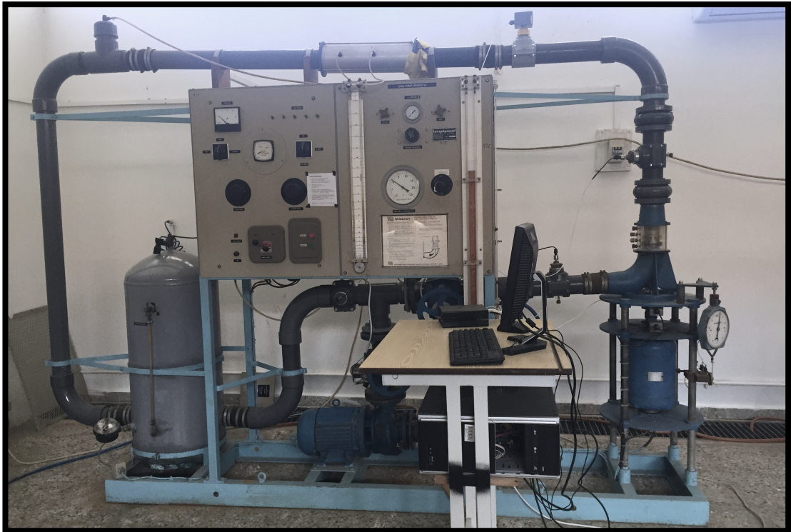
Figure D.1: Axial flow water pump/turbine test Rig H.26
