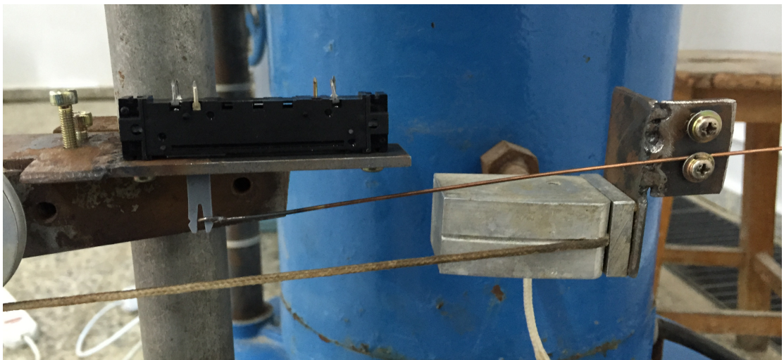
Figure 3.23: Potentiometer fitted on the old torque meter
