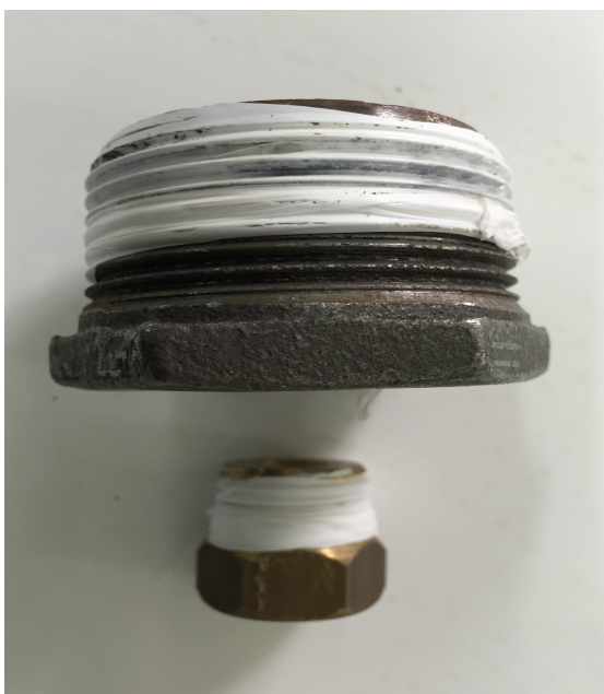
Figure 3.17: Adapters covered with Teflon
