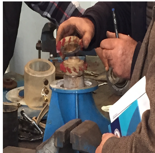
Figure 3.8: Repairing the blades
