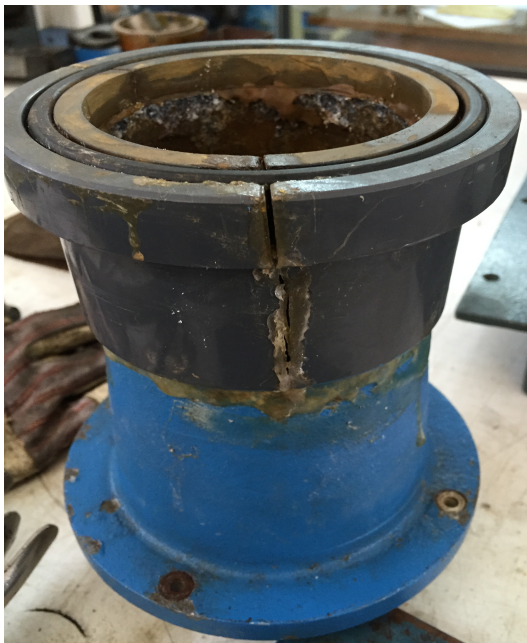
Figure 3.3: Old broken turbine joint
