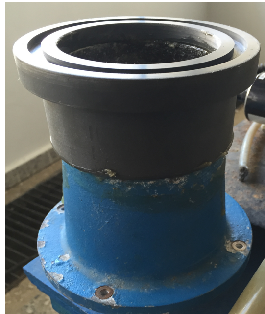
Figure 3.4: Reproduced turbine joint
