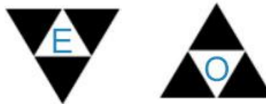
Figure 13: Triangular grid cell types in 3 neighbors case
