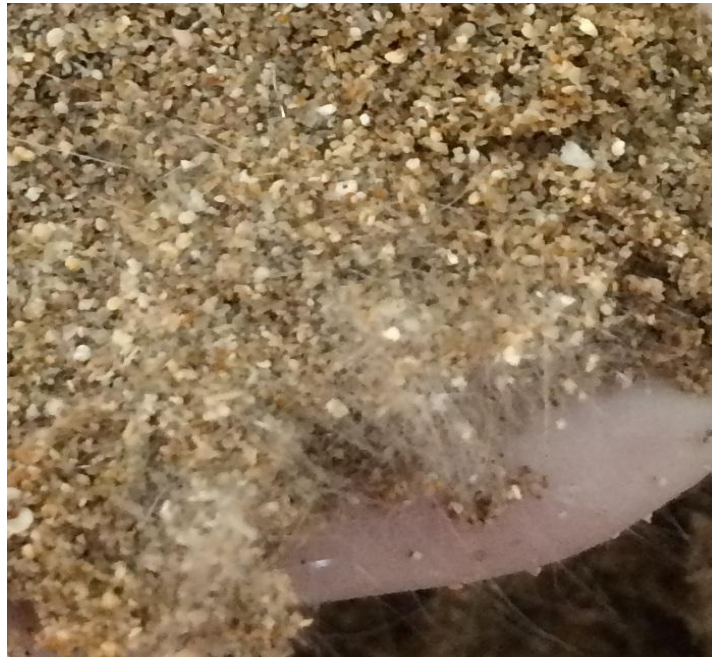
Figure 4.9. Sand reinforced with 1% fibreglass
