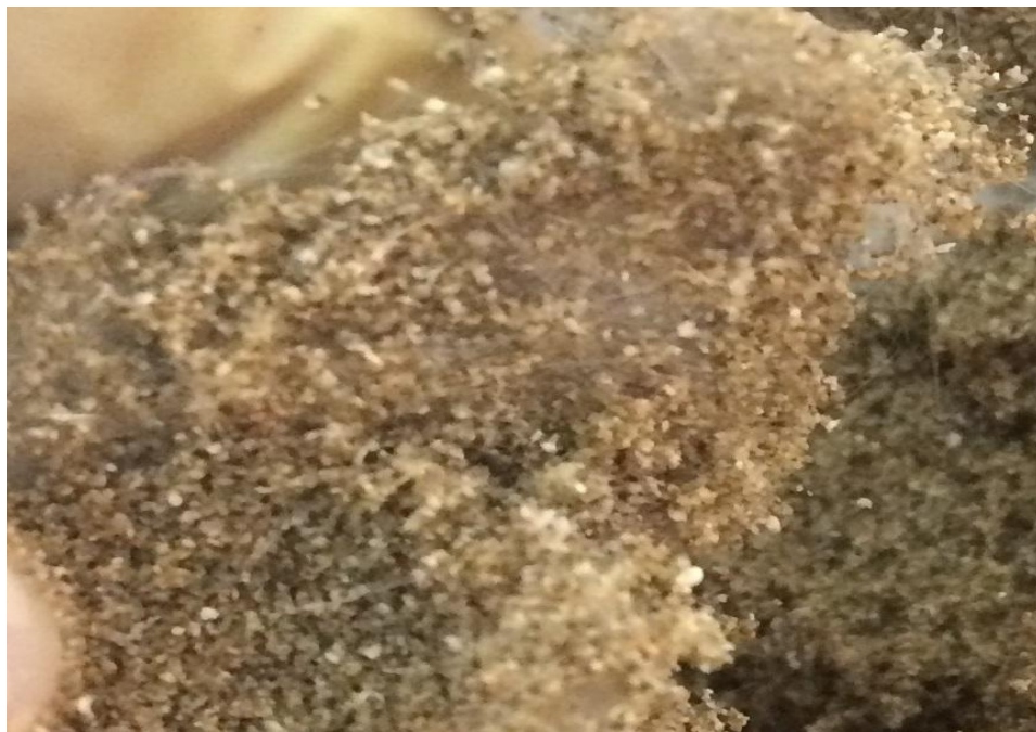
Figure 4.13. Sand reinforced with 1.5% fibreglass
