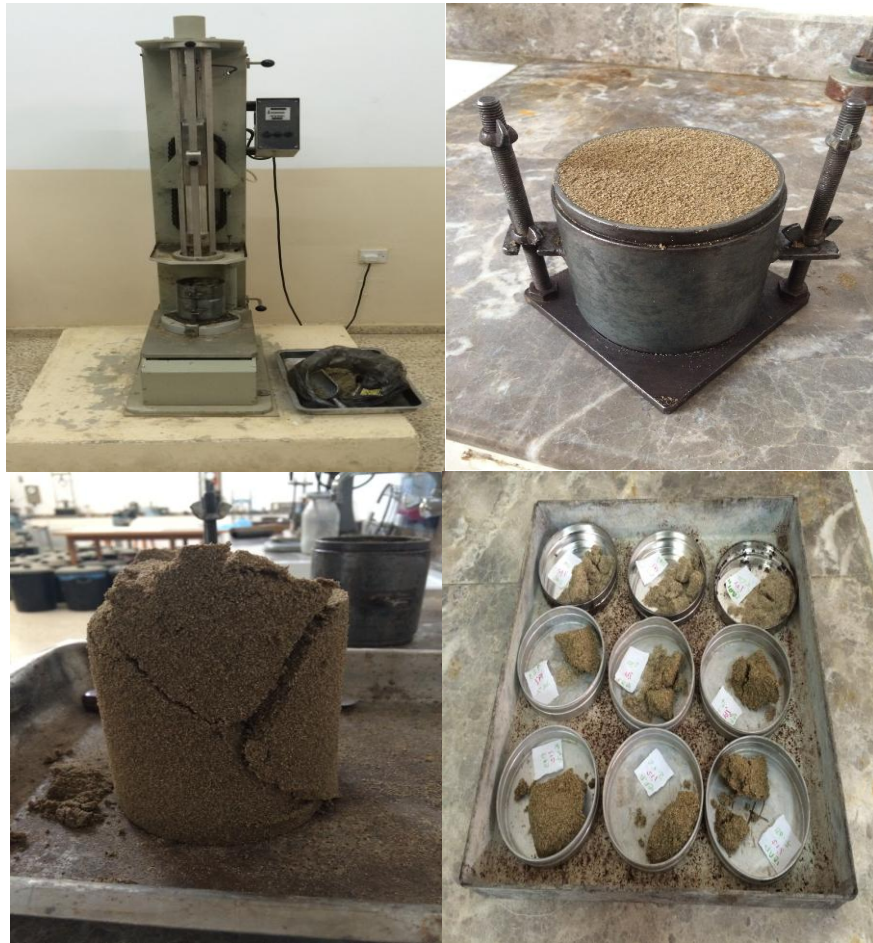
Figure 3.10. Compaction test apparatus and the compacted soil in the mould
