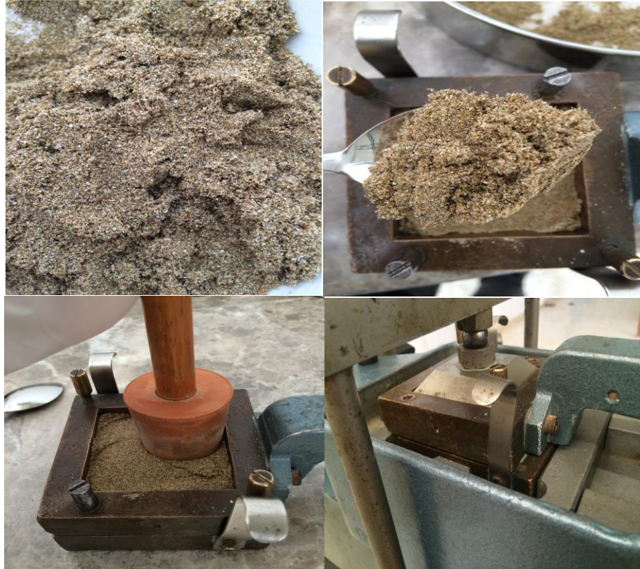
Figure 3.14. Sample preparation for Direct Shear Box test
