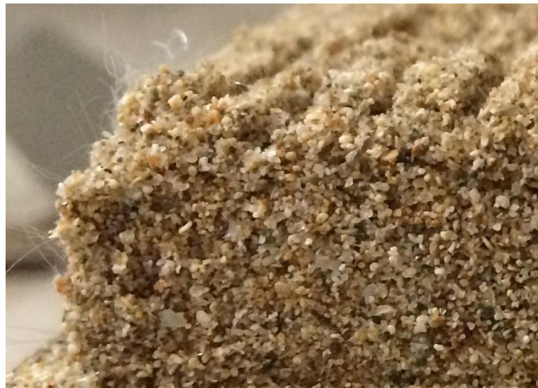
Figure 4.5. Sand reinforced with 0.5% fibreglass
