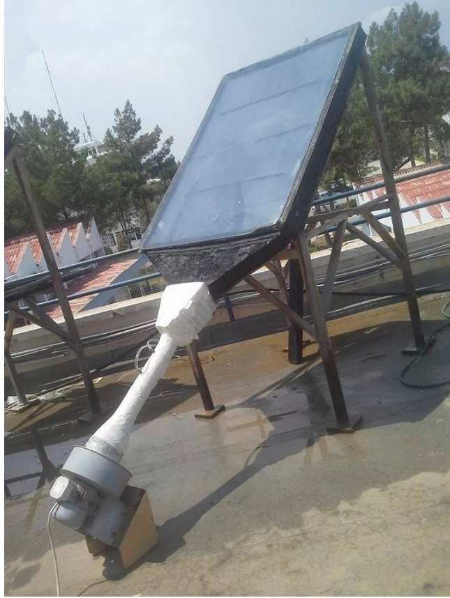
Figure 4.1: Pictorial view of the experimental set up of SAH.
