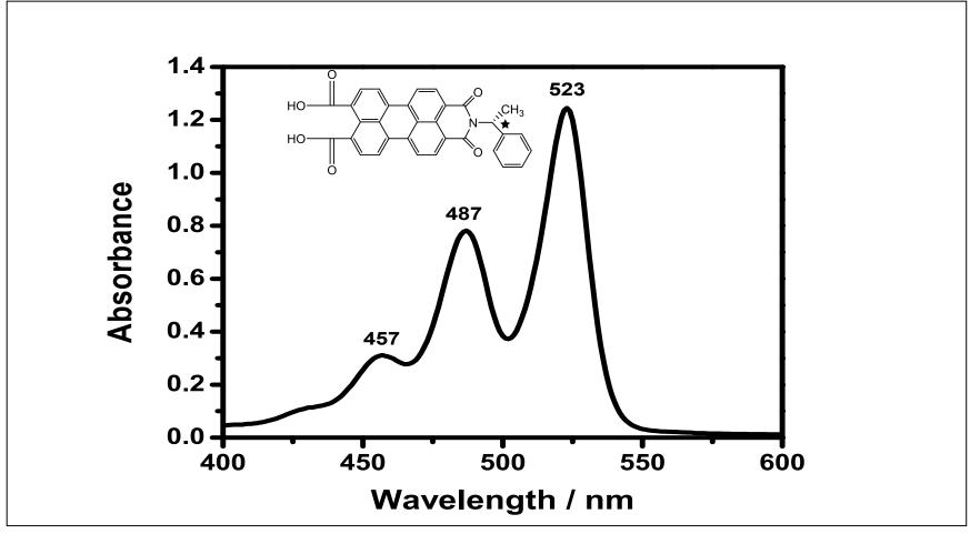
Figure 4.18 Absorption spectrum of R-CPMI in Chloroform
