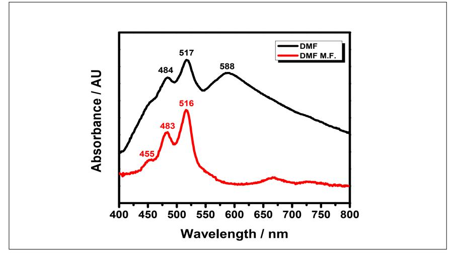
Figure 4. 26 Absorption spectrum of PDA in DMF and DMF microfiltered
