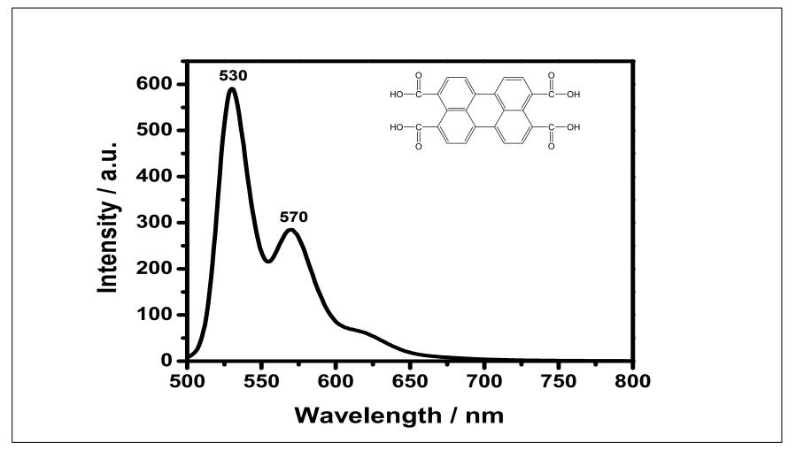
Figure 4. 29 Emission spectrum of PTCA in DMF at  $\lambda_{exc}$  = 485 nm
