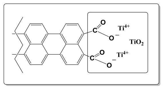
Figure 2. 4 Binding of nanocrystalline TiO<sub>2</sub> with Carboxylic acid group.
