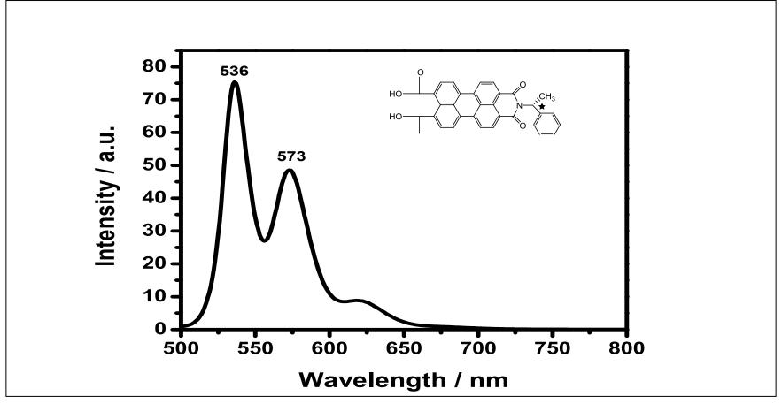
Figure 4.33 Emission spectrum of R-CPMI in Chloroform at  $\lambda_{exc} = 485$  nm
