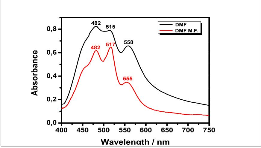
Figure 4.14 Absorption spectrum of PTCA in DMF and DMF microfiltered
