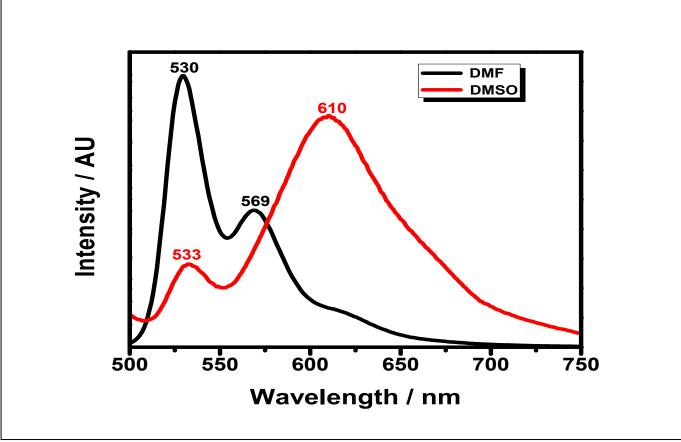
Figure 4.38 Emission spectrum of PDA in DMF and DMSO at  $\lambda_{exc} = 485$  nm
