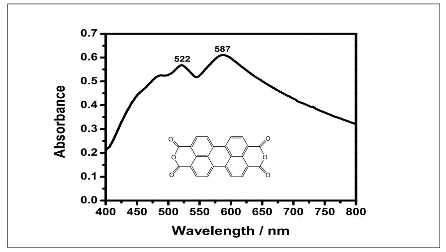
Figure 4.21 Absorption spectrum of PDA in DMSO
