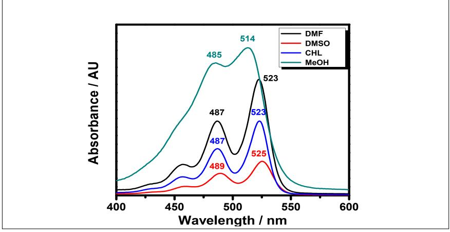
Figure 4.20 Absorption spectrum of R-CPMI in DMF, DMSO, CHL and MeOH
