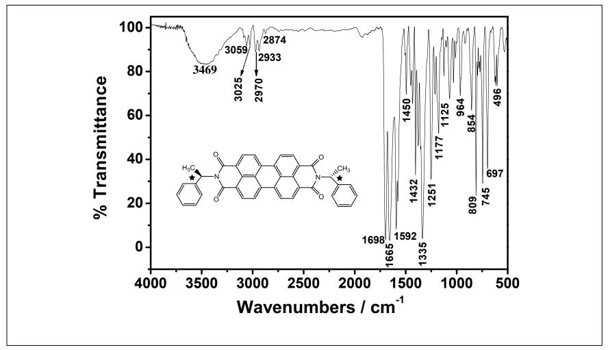
Figure 4. 4 FTIR spectrum of chiral PDI
