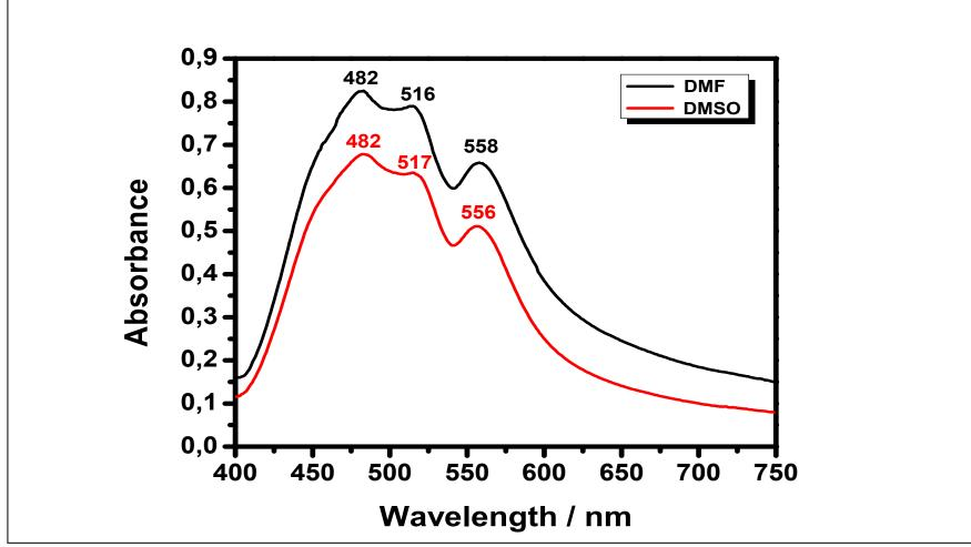
Figure 4.15 Absorption spectrum of PTCA in DMF and DMSO
