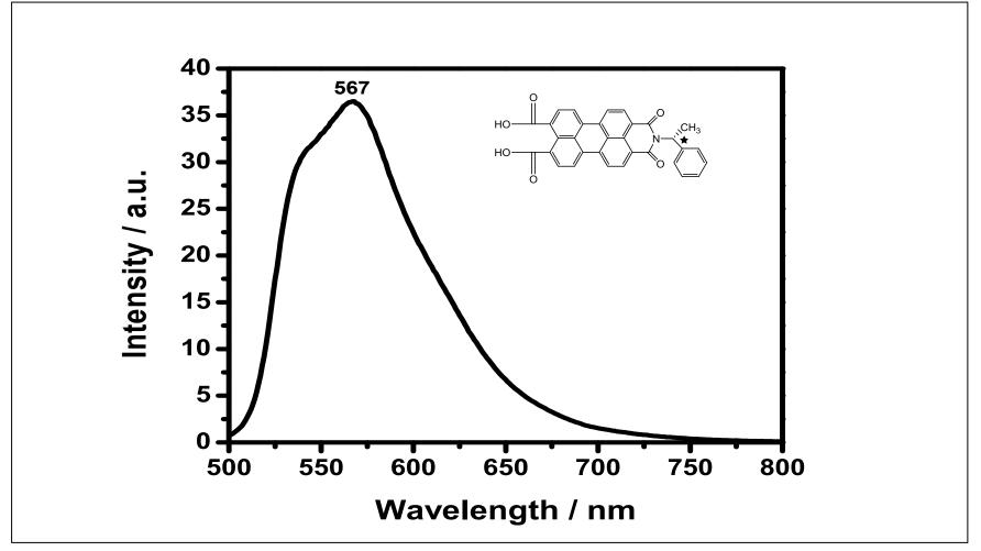
Figure 4.34 Emission spectrum of R-CPMI in MeOH at  $\lambda_{exc} = 485$  nm
