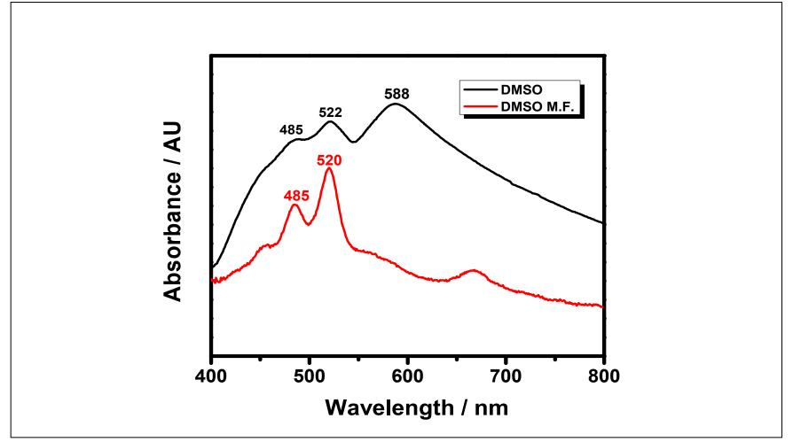
Figure 4.23 Absorption spectrum of PDA in DMSO and DMSO microfiltered
