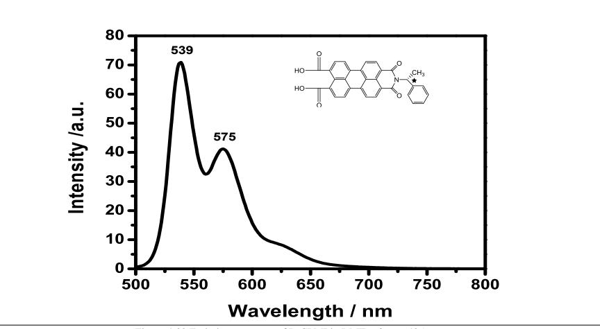
Figure 4.32 Emission spectrum of R-CPMI in DMF at  $\lambda_{exc} = 485$  nm
