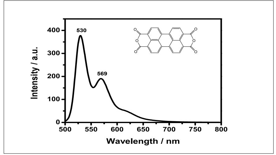
Figure 4.37 Emission spectrum of PDA in DMF M.F. at  $\lambda_{exc} = 485$  nm
