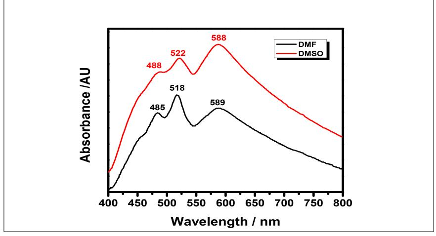
Figure 4. 27 Absorption spectrum of PDA in DMF and DMSO
