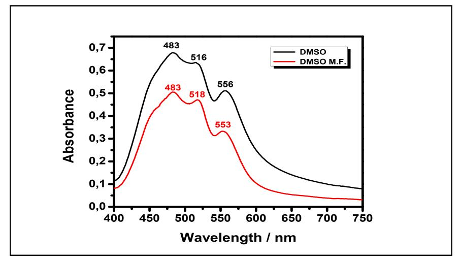
Figure 4.11 Absorption spectrum of PTCA in DMSO and DMSO microfiltered
