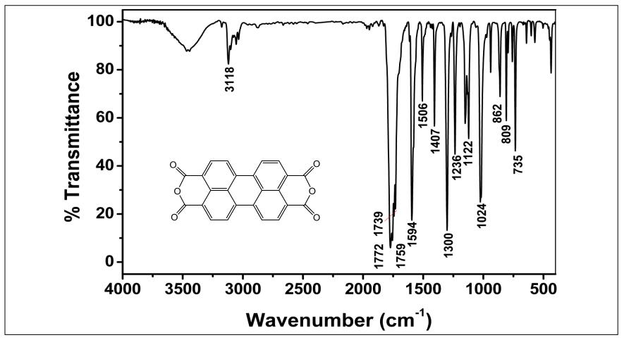
Figure 4.8 FTIR spectrum of PDA
