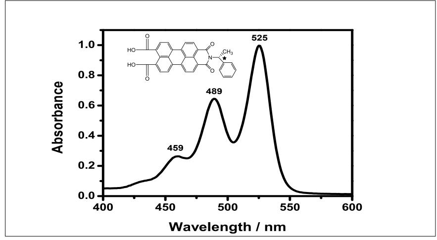
Figure 4.16 Absorption spectrum of R-CPMI in DMSO
