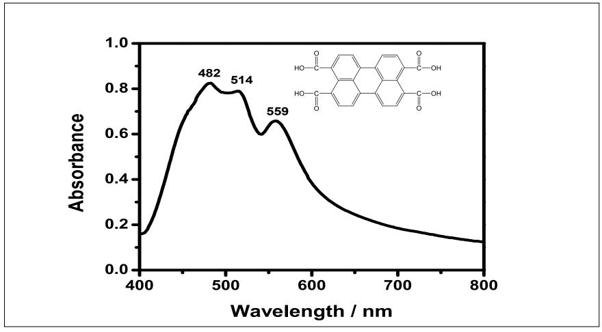
Figure 4.12 Absorption spectrum of PTCA in DMF
