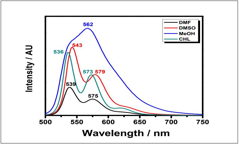
Figure 4.35 Emission spectrum of R-CPMI in DMF, DMSO, CHL and MeOH at  $\lambda_{exc} = 485$  nm
