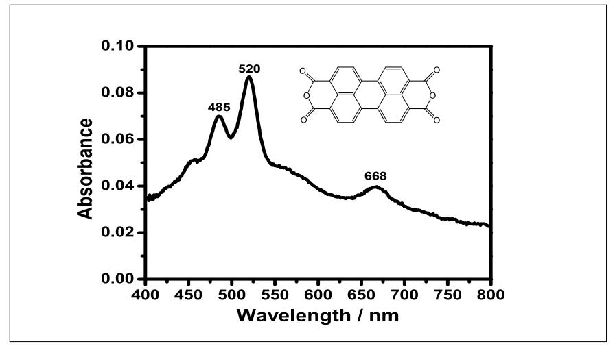
Figure 4.22 Absorption spectrum of PDA in DMSO microfiltered
