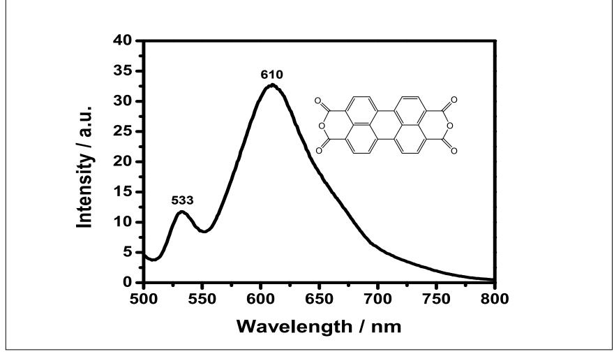
Figure 4.36 Emission spectrum of PDA in DMSO M.F. at  $\lambda_{exc} = 485$  nm
