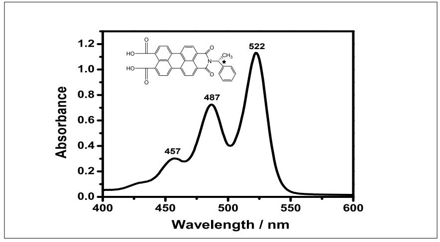
Figure 4.17 Absorption spectrum of R-CPMI in DMF
