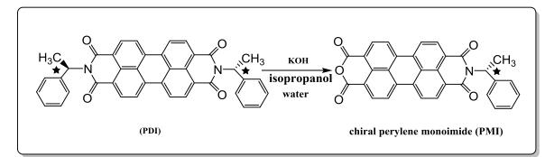
Scheme 3. 4 Synthesis of N-((R)-(+)-1-phenylethyl)-3,4,9,10-perylenetetracarboxylic-3,4-anhydride-9,10-imide (R-PMI).
