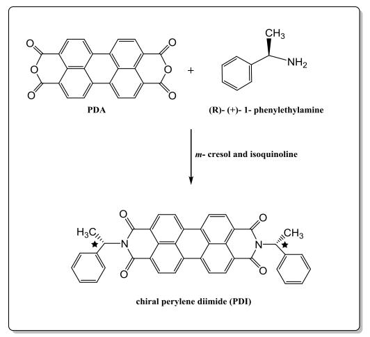
Scheme 3. 3 Synthesis of N,N'-bis((*R*)–(+)–1–phenylethyl)3,4,9,10-perylenenbis(dicarboximide) (PDI) [30].
