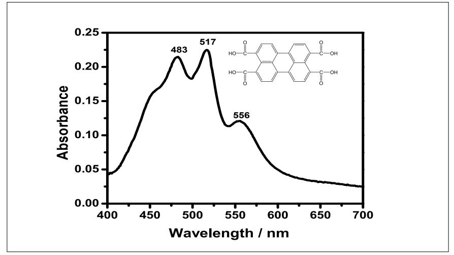
Figure 4.13 Absorption spectrum of PTCA in DMF microfiltered
