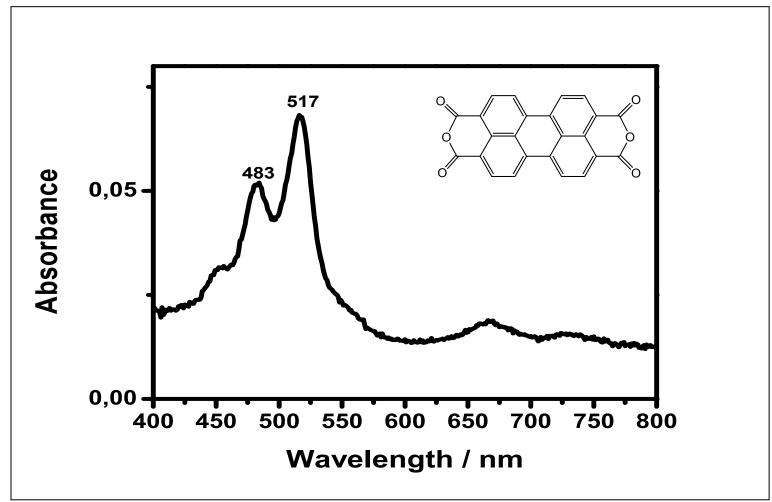
Figure 4.25 Absorption spectrum of PDA in DMF microfiltered
