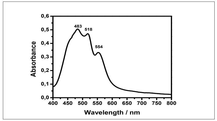
Figure 4.10 Absorption spectrum of PTCA in DMSO microfiltered
