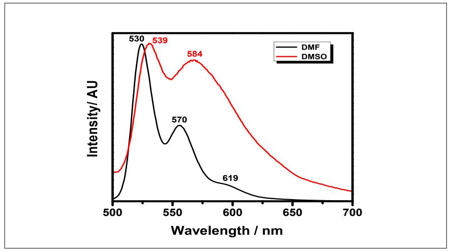
Figure 4.30 Emission spectrum of PTCA in DMF and DMSO at  $\lambda_{exc}$  = 485 nm
