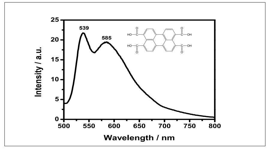
Figure 4.28 Emission spectrum of PTCA in DMSO at  $\lambda_{exc} = 485$  nm
