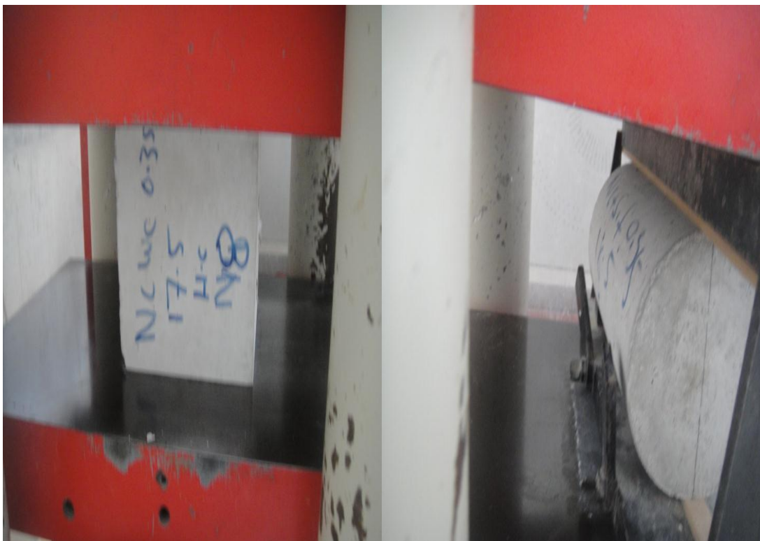
Figure 3.8. Compressive and tensile testing, respectively
