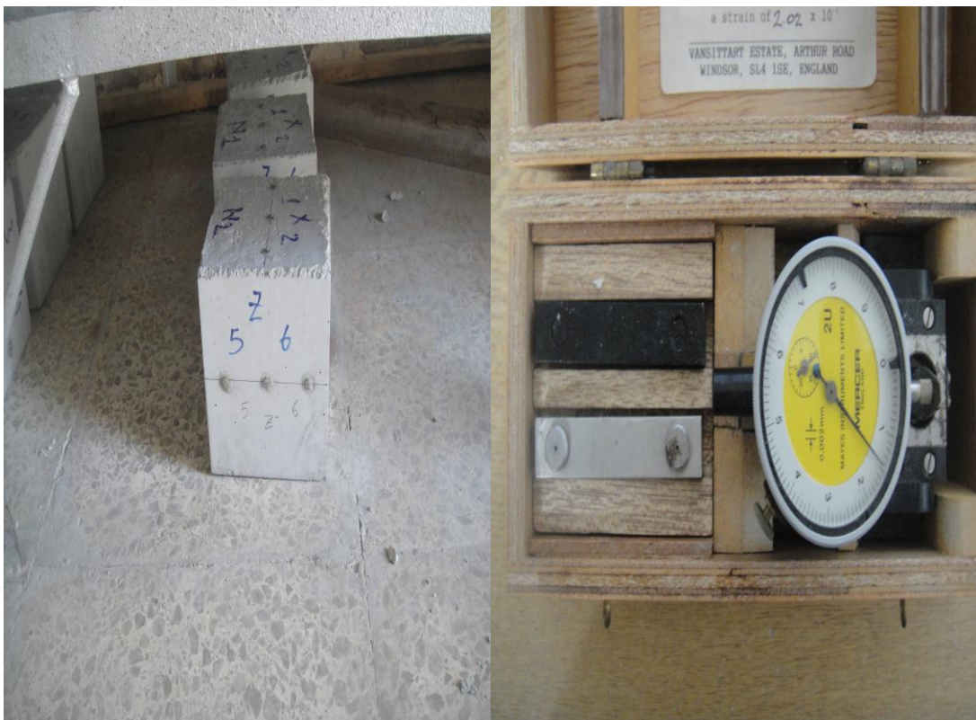
Figure 3.9. Length change measurement with time by using shrinkage pins placed in three directions
