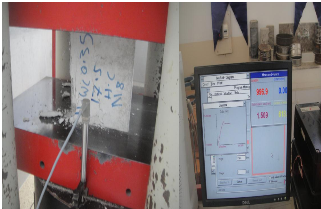
Figure 3.10. Determination of stress-strain diagrams subjected to compressive stress
