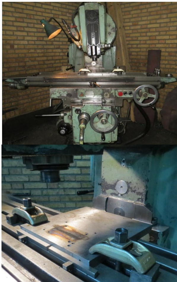
Figure 3.4 Machine and fixture used in FSP.
