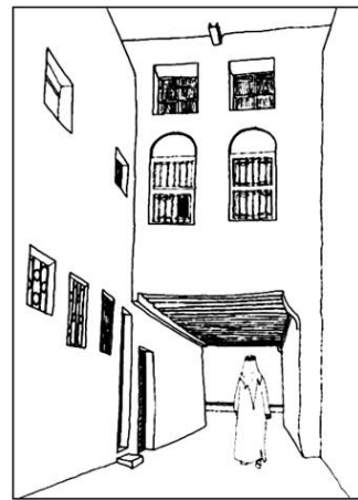
A SABAT IN HOFUF, SAUDI ARABIA. PALM TREE TRUNKS ARE USED FOR THE MAIN STRUCTURE FOR SUPPORT.
