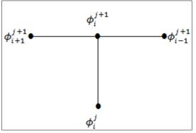
Figure 1. Computational molecule for BTCS
