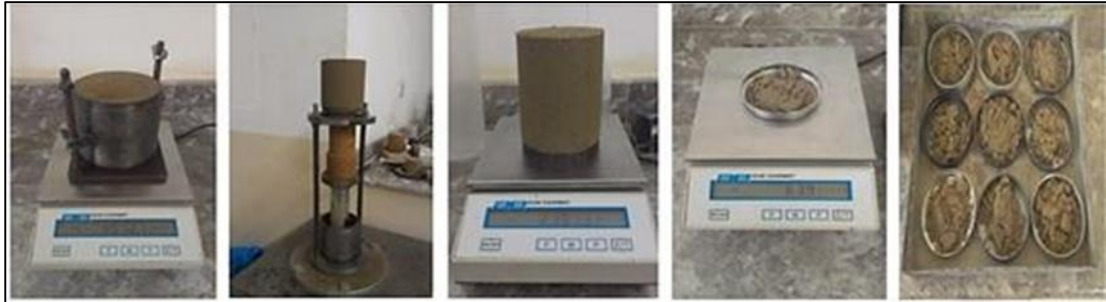
Figure 21: (Left to right) Weighting, extracting and sampling of the sand
