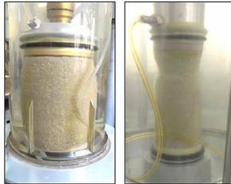
Figure 46: Deformation of soil sample in compression & extension (Rocker, 1968)
