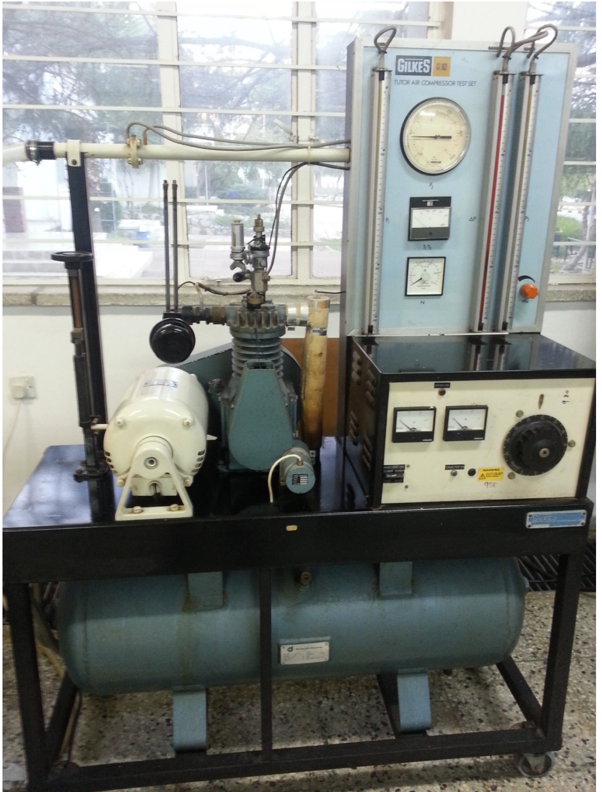
Figure 4.6. Air compressor and controlling unit
