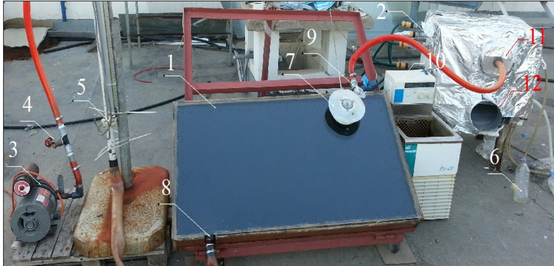
1.Humidifier, 2.Condenser, 3. Compressor, 4. Bypass valve, 5.Orifice meter, 6. Fresh water collector, 7.Pyranometer, 8.Humidifier air inlet, 9.Humidifier air outlet, 10.Cooler, 11.Condenser air inlet, 12.Condenser air outlet.
