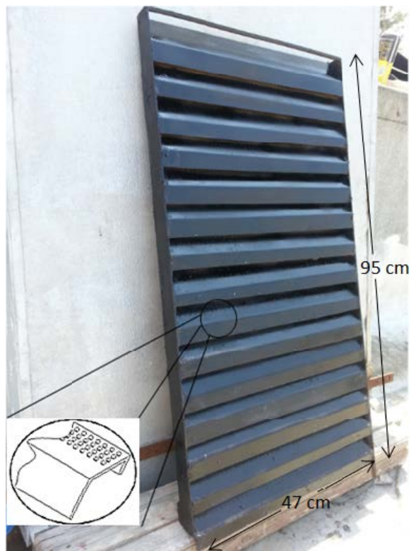
Figure 5.4. A stack of Inverted sieves (heat absorber and bubble regenerator)
