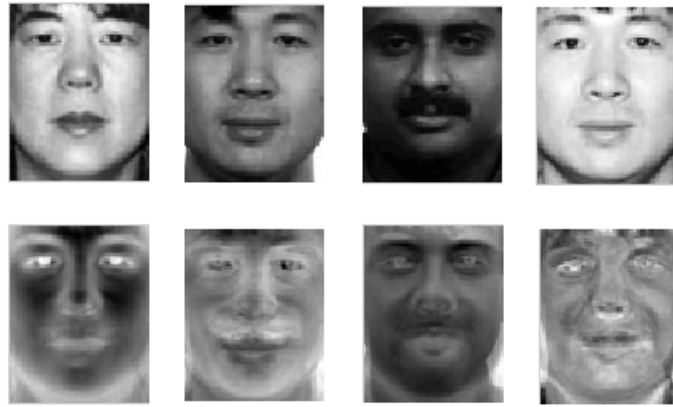
Figure 6. Original images (the first row), and the corresponding Eigenfaces obtained (the second row)
