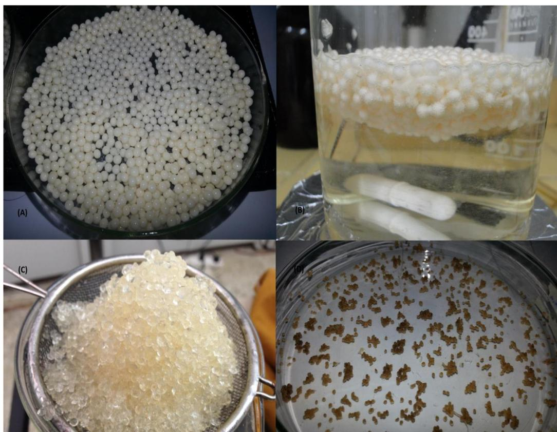
Figure 5.(A)Chitin beads with  $\text{CaCO}_3$ , (B) Chitin beads in 3M HCl, (C) Porous Chitin Beads before dry, (D) Porous Chitin Beads after drying
