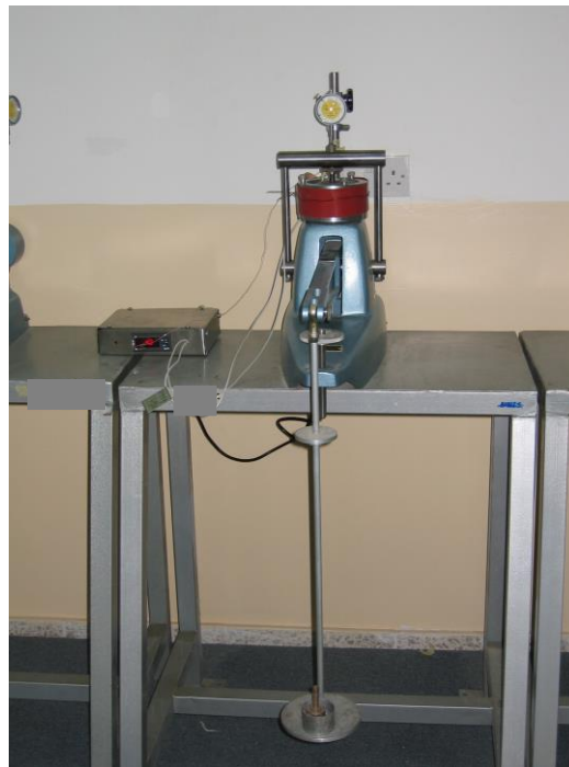
Figure 3.5 The modified consolidometer with temperature controller
