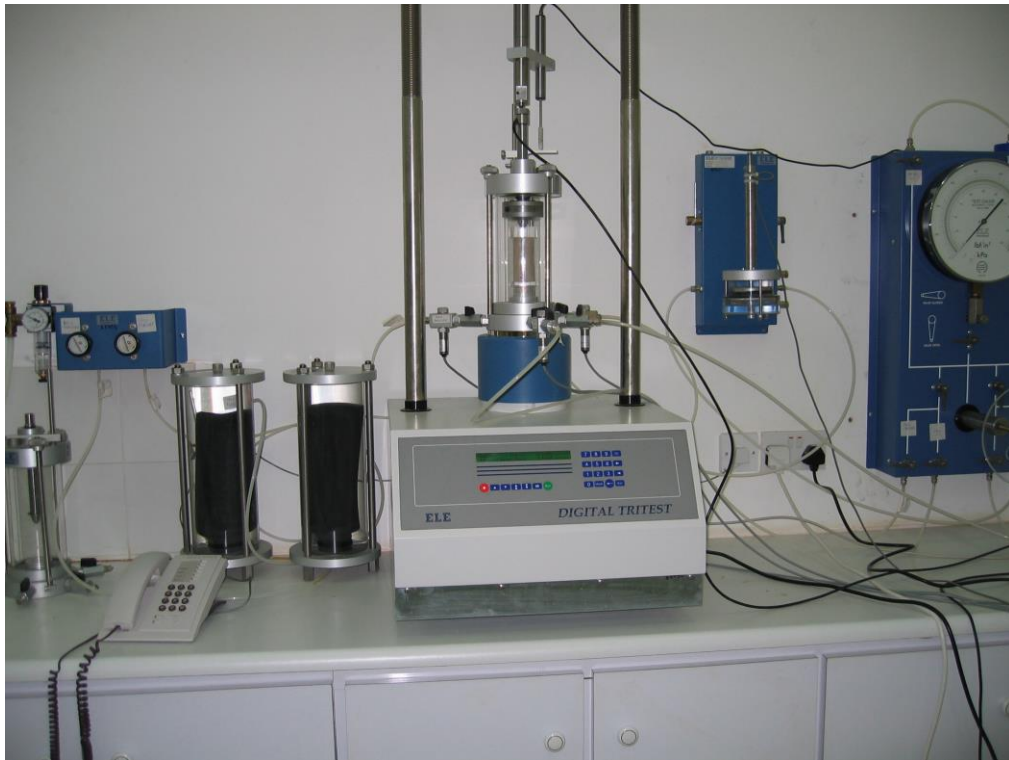
Figure 3.7 Consolidated undrained triaxial test setup
