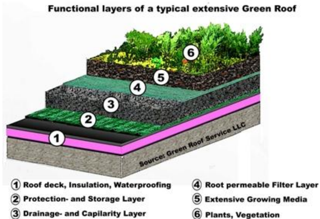
Figure 2.1: Extensive Green Roofs Layers [3]
