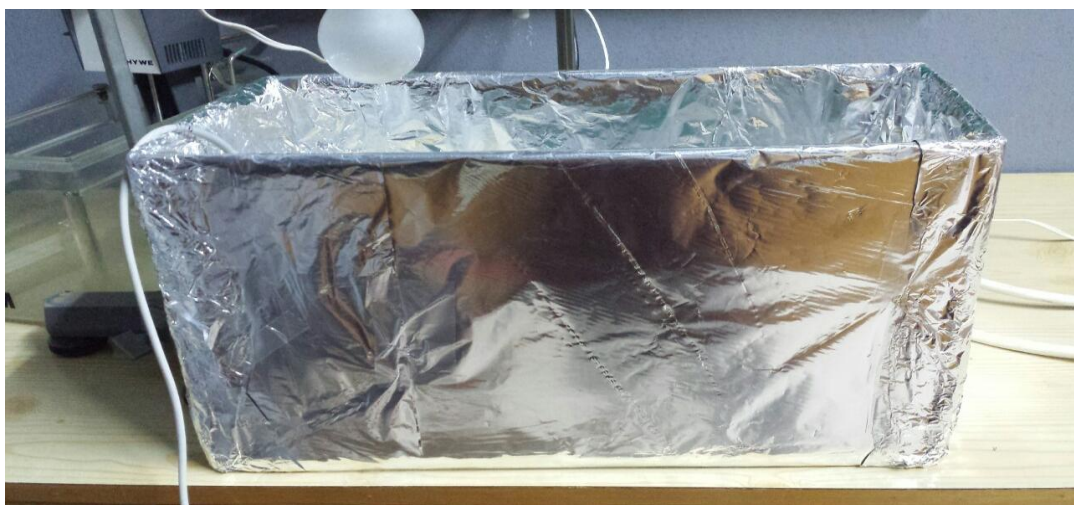
Figure 3.2. Faraday cage is constructed from aluminum foil, electric bulb was used to keep the temperature at 37°C
