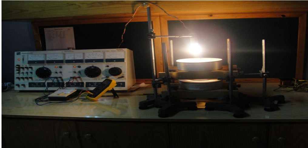
Figure 4.2. Electromagnetic field exposure system the sample was placed at the midpoint of the two Helmholtz coil. Electric bulbs was used to keep the temperature at 37°C
