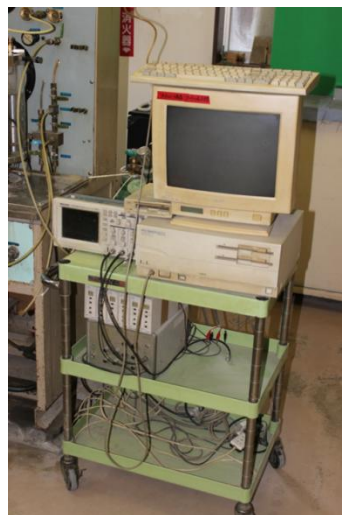
Figure 5.10: V_S and V_P measurement system
