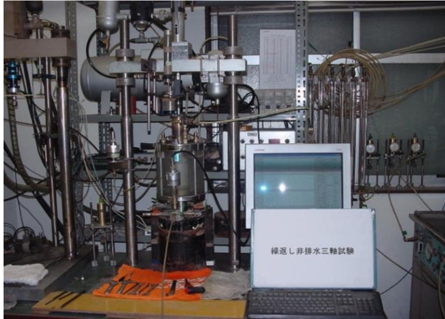
Figure 5.5: Pneumatic cyclic triaxial test apparatus used for undisturbed samples in the laboratory of Kiso-Jiban consultants Co. Ltd
