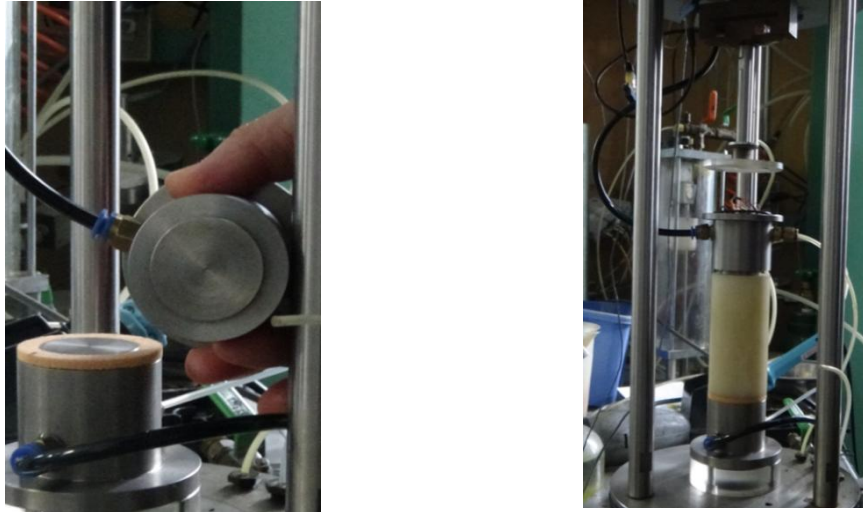
Figure 5.8: The top cap and pedestal of triaxial cell
