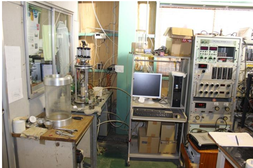
Figure 5.4: Hydraulic cyclic triaxial test apparatus used for reconstituted samples in The laboratory of Kiso-Jiban consultants Co. Ltd
