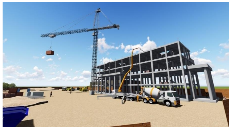
Figure 27: 3D Construction Jobsite Organization Model
